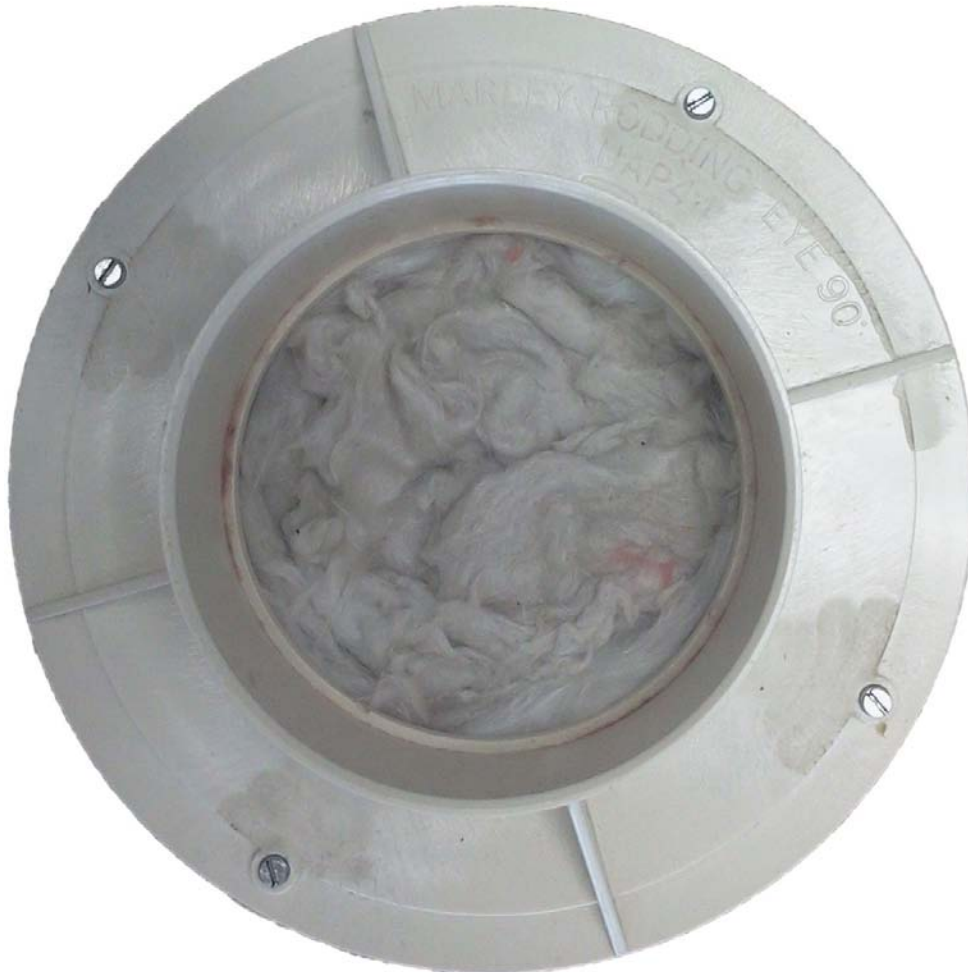
Figure 27: Placing fibrous material on the loudspeaker cone smooths the frequency of response
