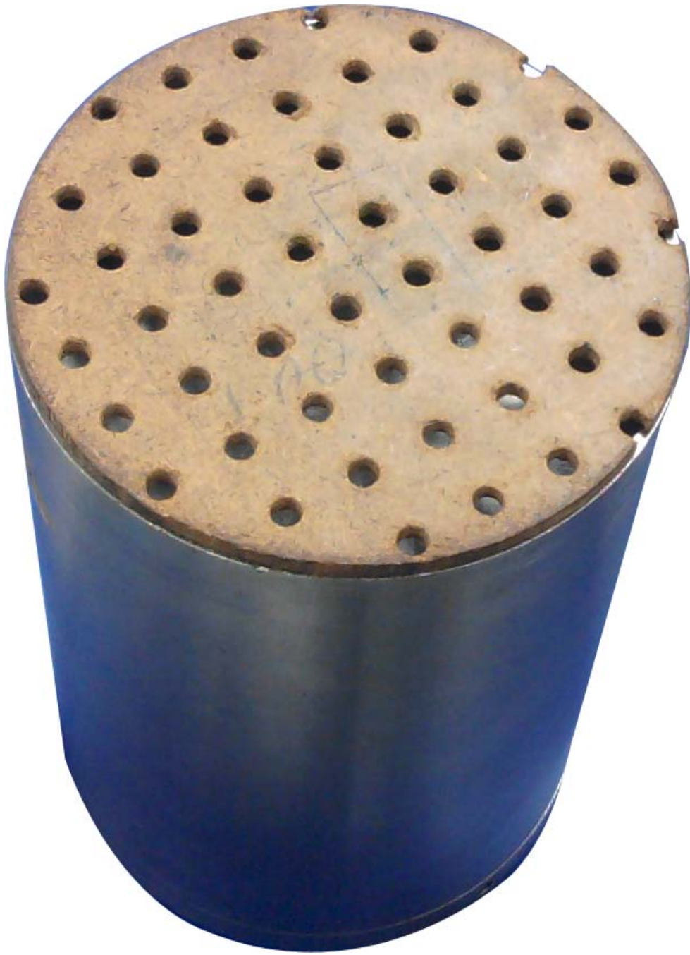
Figure 65: The Helmholtz resonator created with the sample holder and a perforated hardboard.
