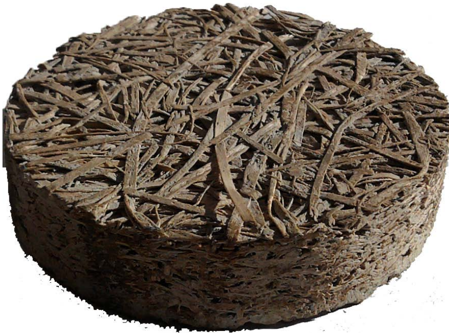
Figure 62: Haraklith wood fibreboard sample used in testing.
