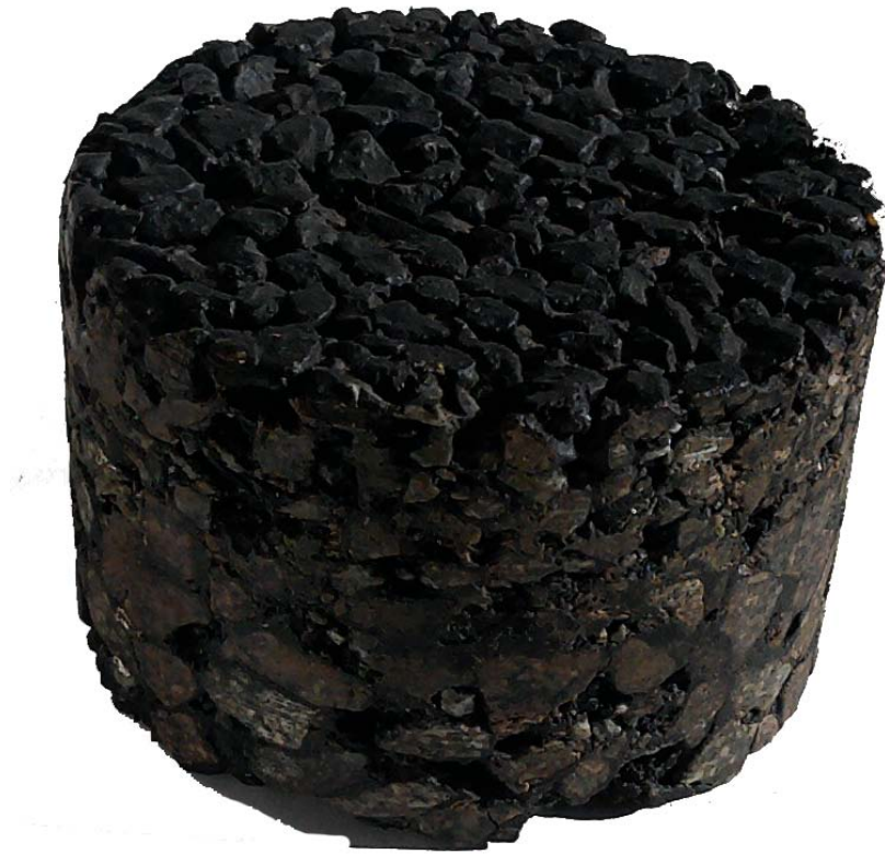
Figure 53: TwinLay asphalt sample.
