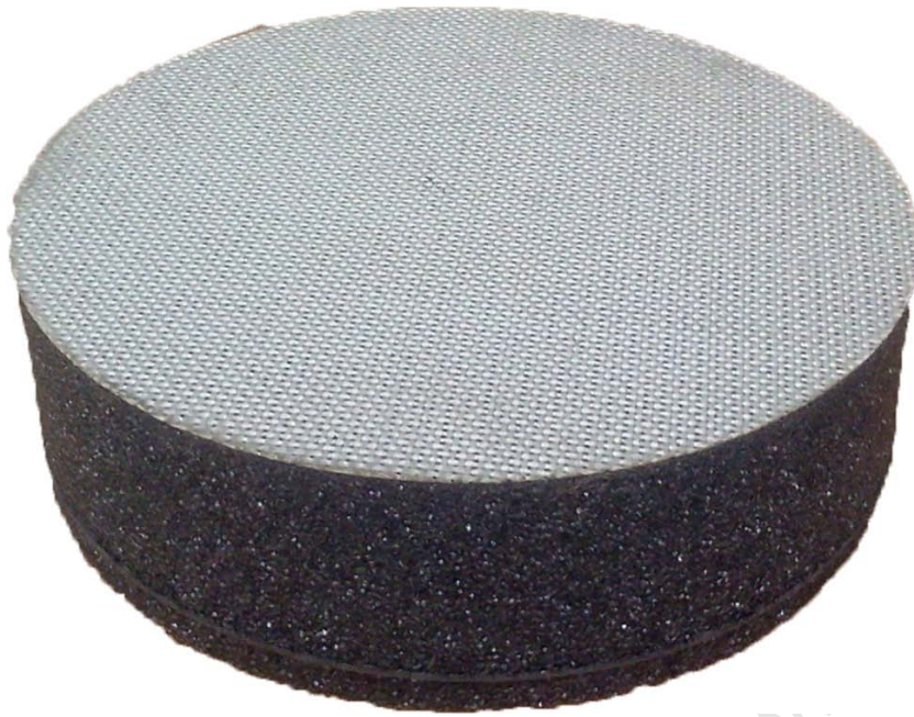
Figure 59: Polyurethane foam sample #1, an open pore foam sample with a 1 mm rubber panel embedded inside of it.
