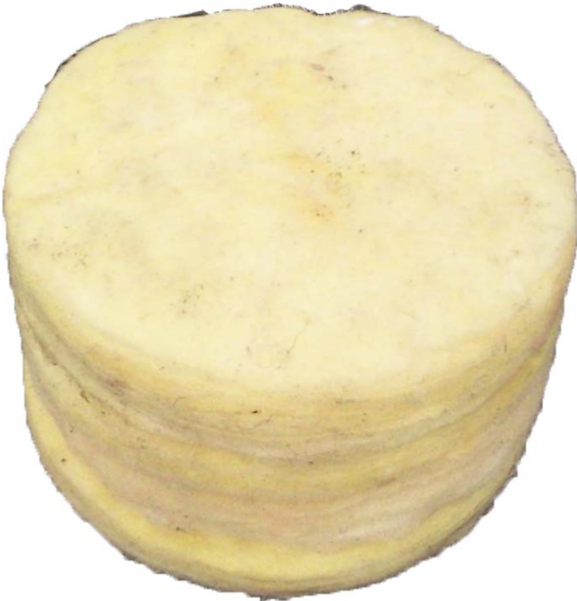
Figure 56: 60mm of glass fibre sample used in testing.
