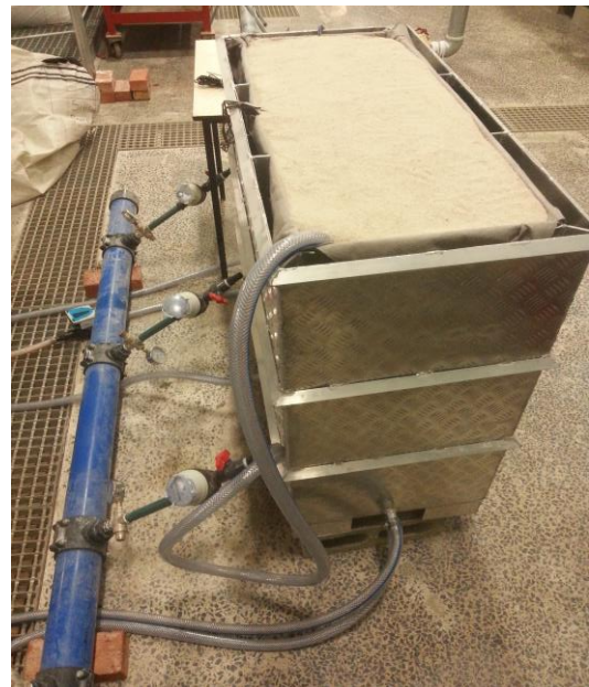
Figure 3-8 : Delivery pipe connected to hose
