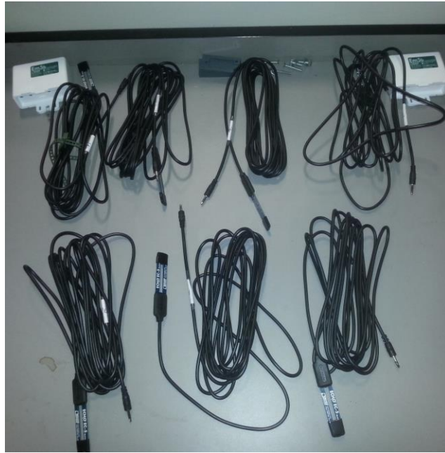
Figure 3-13: 7 EC-5 sensors and 2 EM-5 loggers used in the experiments
