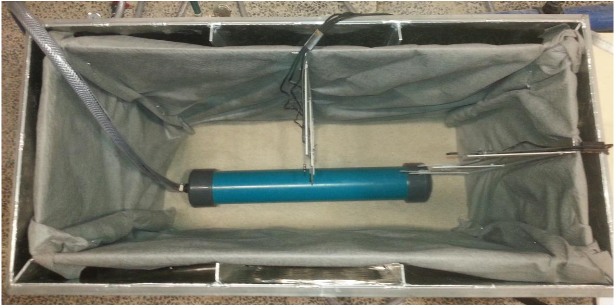
Figure 3-9: Pipe Sample connected to detachable hole through end cap
