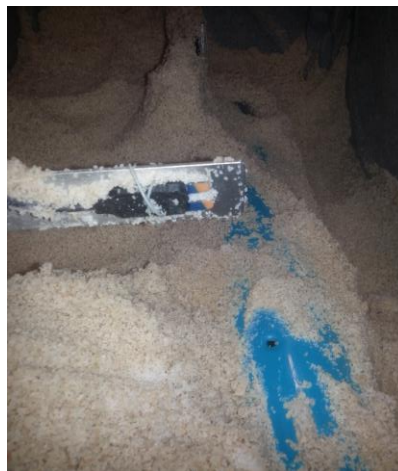
Figure 4-24: Damaged sensor above leak
