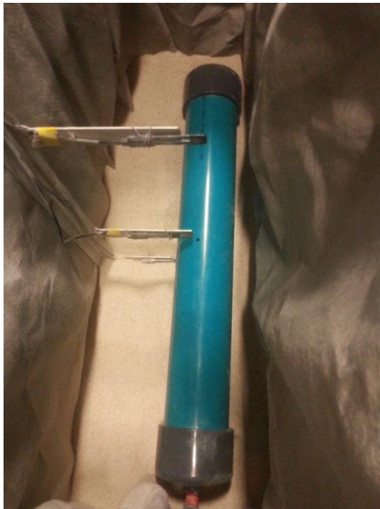
Figure 3-27: Upward pointing Leak
