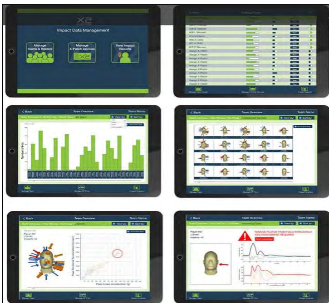
Figure 2: Example of the data display provided by the IMS, with data including, but not limited to, xPatch player assignment and charge levels, and number, location, and severity of impacts recorded per xPatch (X2Biosystems Inc., 2013).
