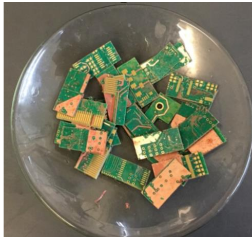
Figure 31 Solder mask layer on PCBs in experiment 4 after solvent swelling and potassium permanganate oxidation, before leaching
