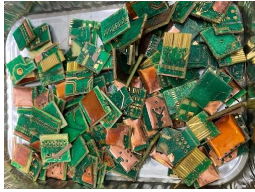
Figure 37 i) Experiment 7 -Cut PCBs after swelling with NMP ii) Experiment 8 Cut PCBs after swelling with solvent B
