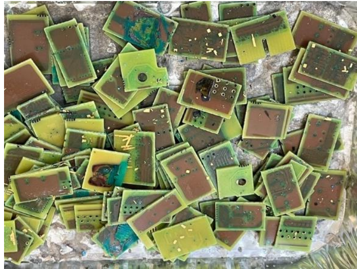
Figure 35 Untreated PCBs in experiment 6 after leaching with waste etchant
