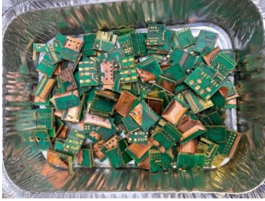
Figure 37 i) Experiment 7 -Cut PCBs after swelling with NMP ii) Experiment 8 Cut PCBs after swelling with solvent B
