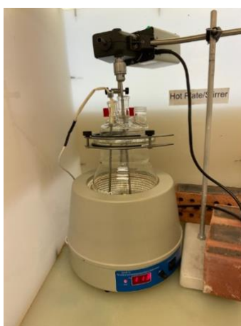
Figure 17 Solvent swelling reactor setup
