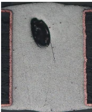
Figure 25 Coupon D 50X magnification view of plated through hole
