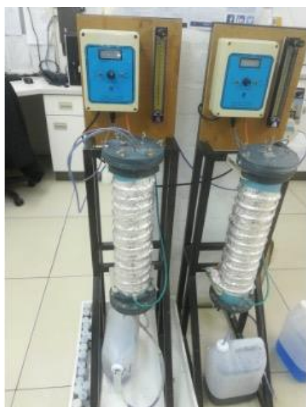
Figure 18 Leaching column configuration
