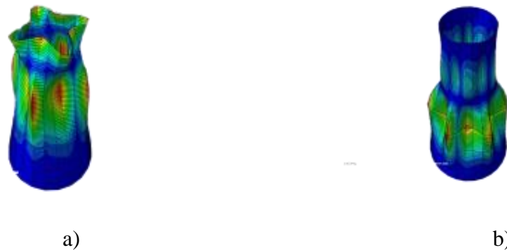
Figure 2-37: Buckling mode shapes [(reproduced from (Ponath & George, 2016)]
