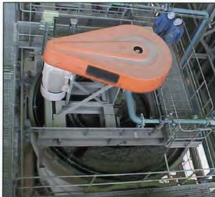
Figure 1.3: Typical Mechanically Agitated Flotation Cell
