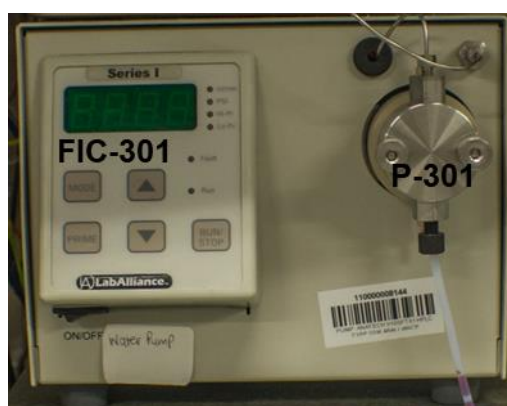
Figure 4.40: Flow controller and indicator for water, accessible on bottom front panel of reactor system
