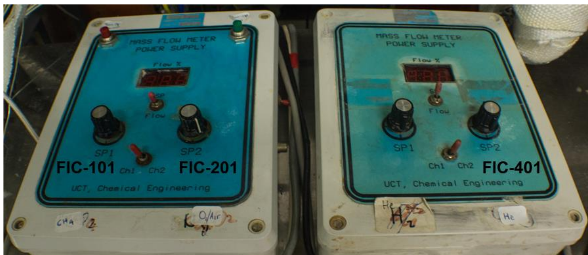
Figure 4.39: Flow control modules and indicators for methane, oxygen and helium, accessible from front platform of reactor system
