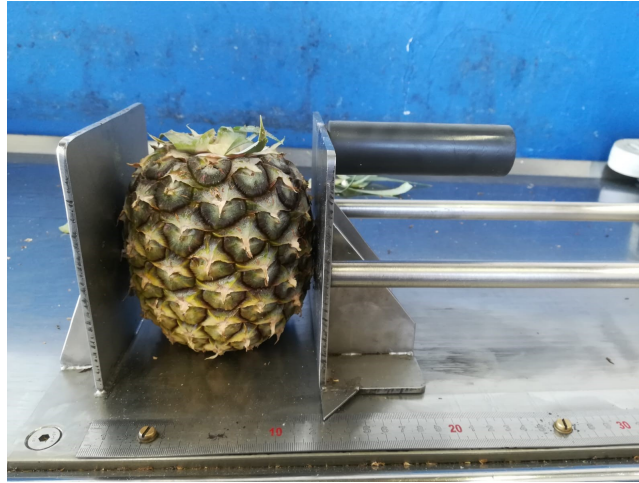
Figure 5.3: Calliper system used for manual measurement of pineapples for size determination evaluation.
