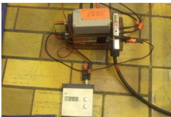
Figure 4-4: PD test configuration showing test equipment and a typical result screen.
