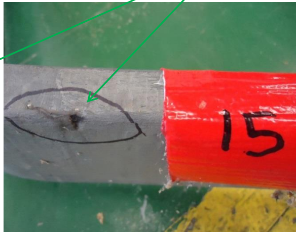
Figure 4-7: HV test configuration with 50 kV test set and fault location of some failed bars
