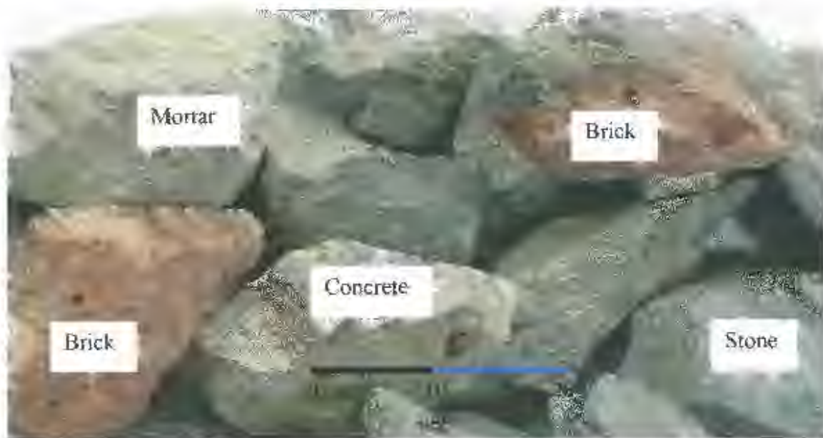
Figure 4.5: Particle shape and texture of the 19 mm RCA
