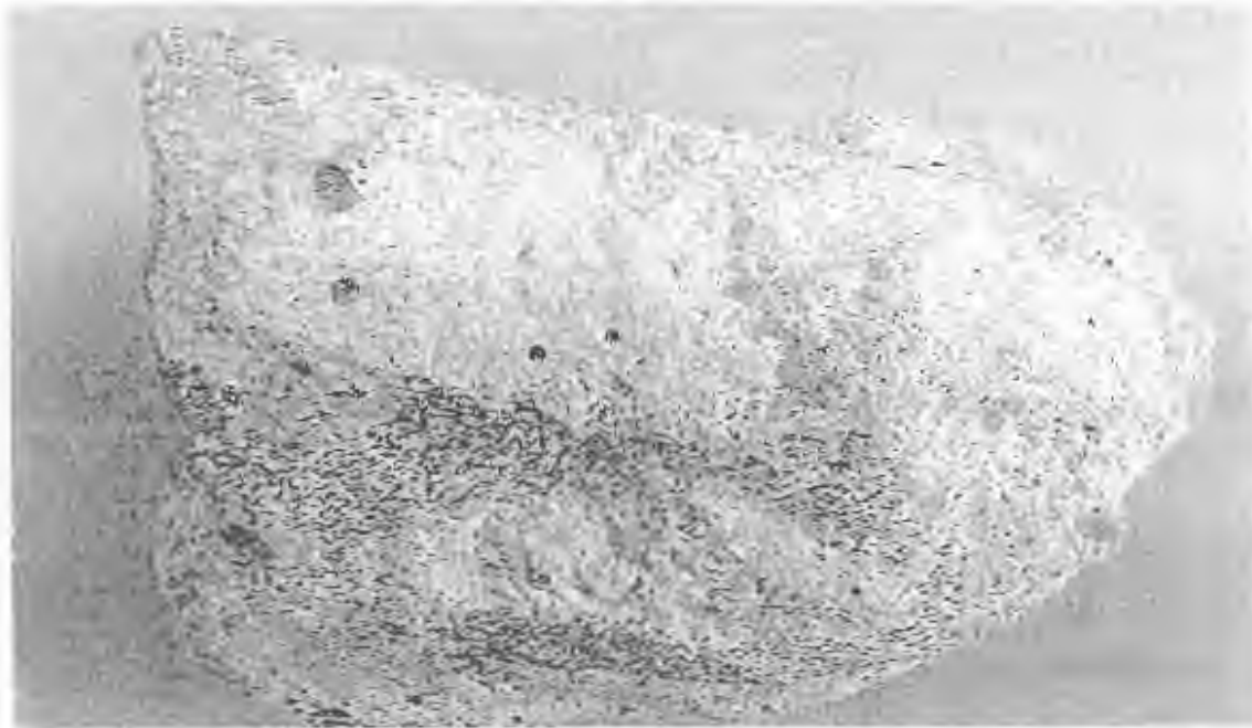
Figure 2.4: RA showing rough and porous surface texture (Alexander et al 2002)
