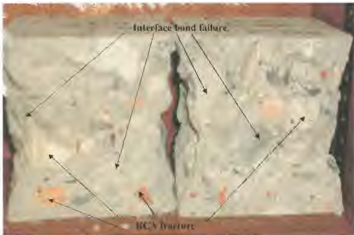
Figure 6.2: Mode of failure of crushed cubes
