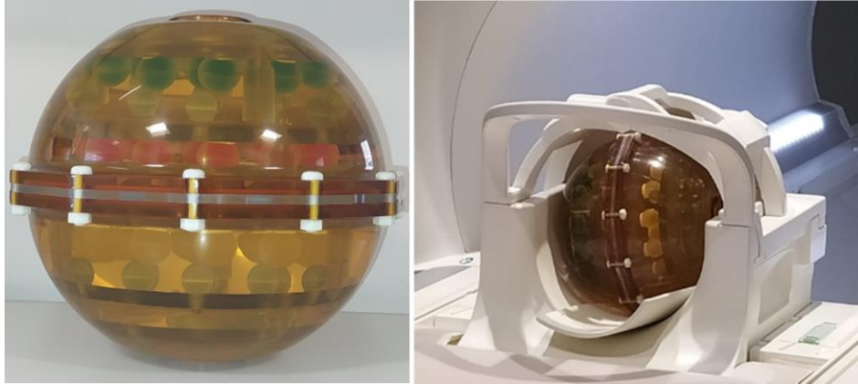
Figure 2-4 High Precision Devices (HPD) system phantom model 130, which contains 5 plates, 57 fiducial spheres and 2 wedges, and its placement in the 20-channel head/neck coil.
