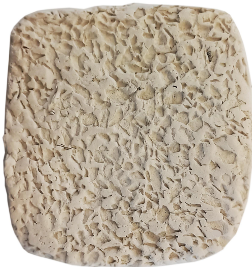
Figure 18. Auwal Mosque's front wall pressed clay negative texture
