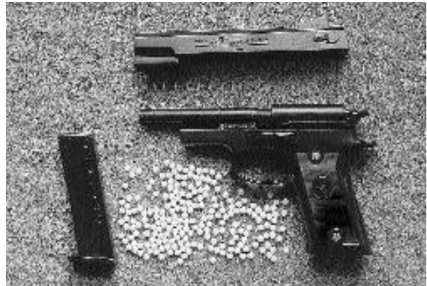
Fig. 2. Disassembled gun with magazine and projectiles. (Note that the spring seen here is not the internal spring mechanism, which powers air propulsion of the projectile.)
