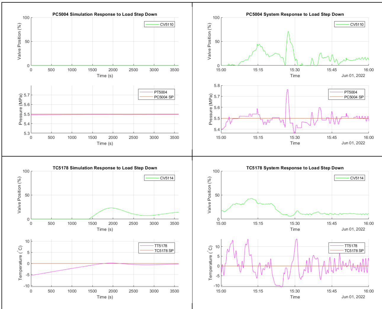
Figure 27: Response of designed controllers in simulation (left) and manually tuned controllers in the physical system (right) in response to a step down in load
