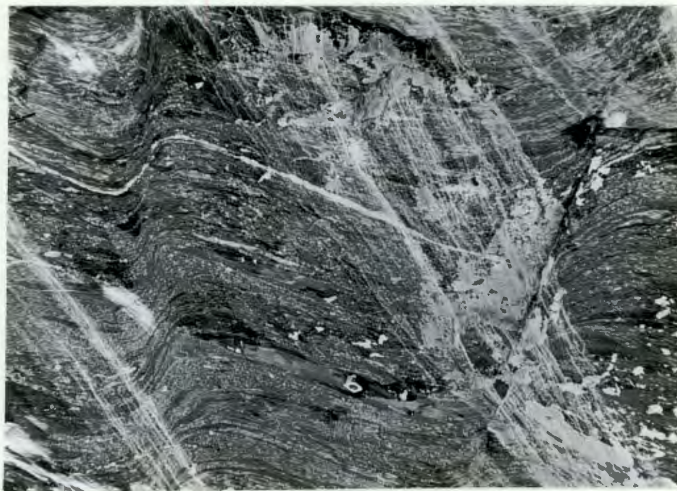
Plate 16. Asymmetric F_5 in interbanded megacrystic granite and paragneiss (Altdorn); a foliation ( s_5 ) is commonly developed along the short limb.
