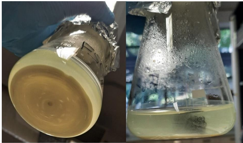
Figure 6-3 Observed precipitation in flasks containing tin, postulated to be \text{SnO} (Brandl et al. 2001; Bryan et al. 2015; Ilyas et al. 2007).
