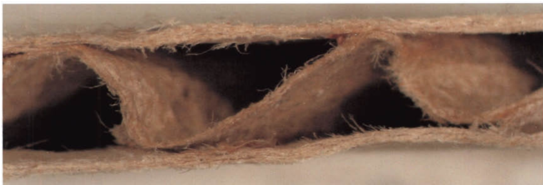
Figure 5.32: Cross-section of a buckled panel showing transverse shearing.
