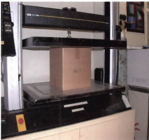
Figure 4.6a: The BCT of a corrugated box.
