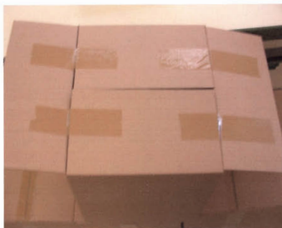
Figure 4.7: Sealing of the inside flaps prior to BCT.
