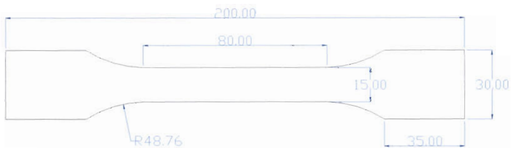
Figure 4.3: Corrugated board tensile specimen dimensions (mm).
