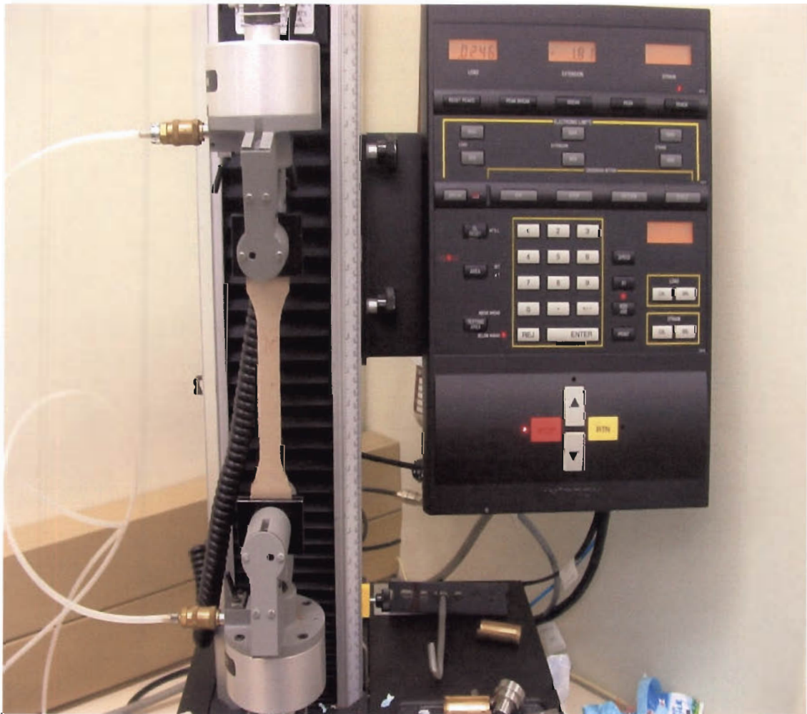
Figure 4.4: A corrugated board tensile test being performed on an Instron 4444 universal tester at Nampak R&D.
