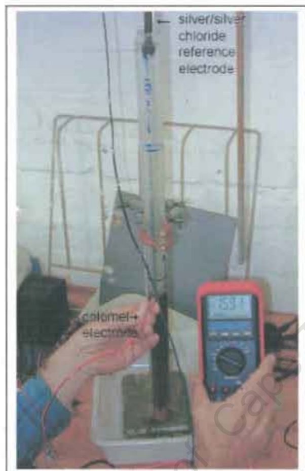
Figure 3.1. Measurement of the redox potential from a sediment core taken from the site of a benthic flux deployment.
