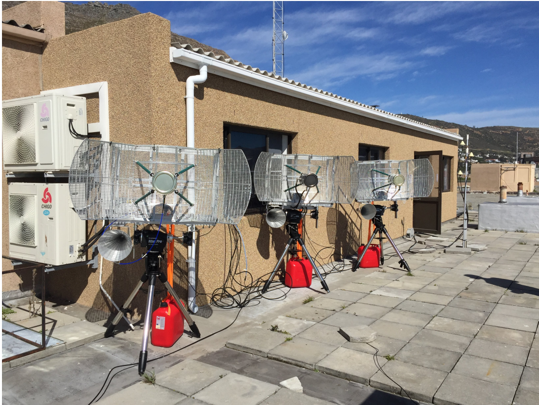
Figure 5.2: NeXtRAD monostatic and passive antennas (left) and GPS antenna mount (right). Set in a quasi-monostatic bistatic geometry.
