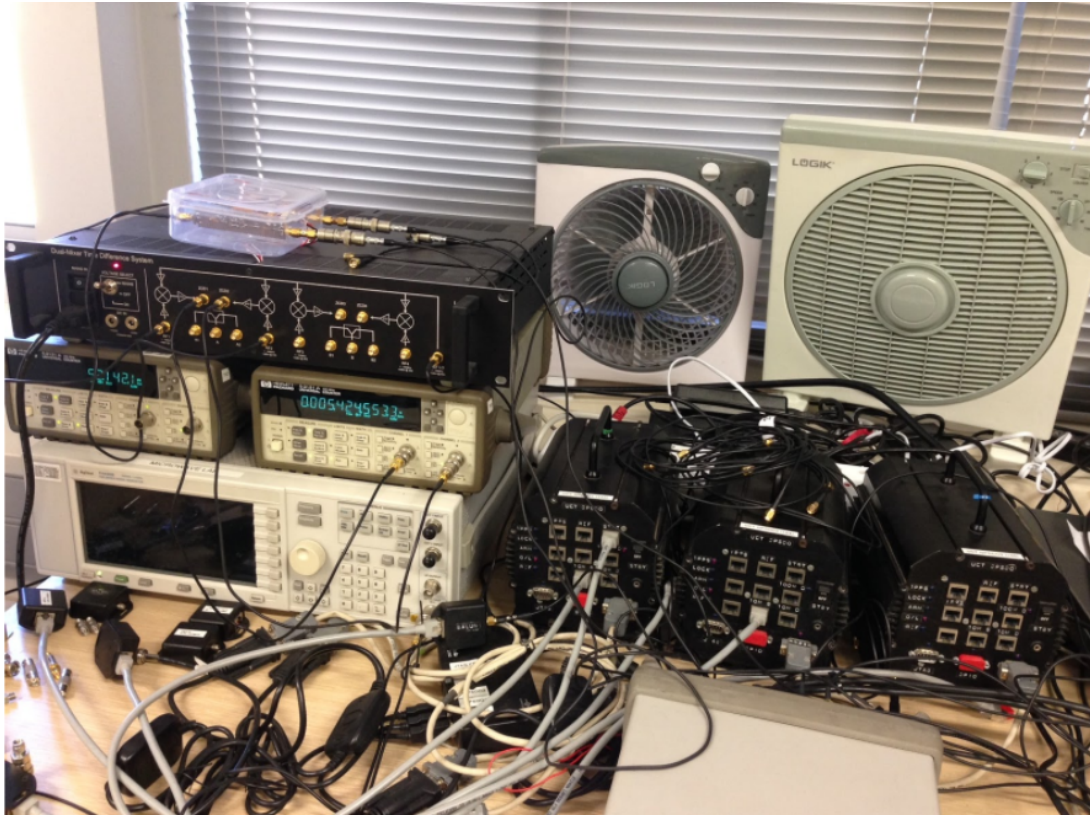
Figure 4.3: WR and GPSDO test bench. Left (from bottom up): E4400B synthesiser, HP53131A TICs, UCT DMTD, fine delay filters. Right: UCT GPSDOs
