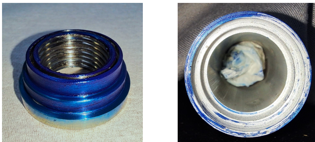
(a) The output flange with engineer's blue applied (b) End view of the blue present on the output trap
