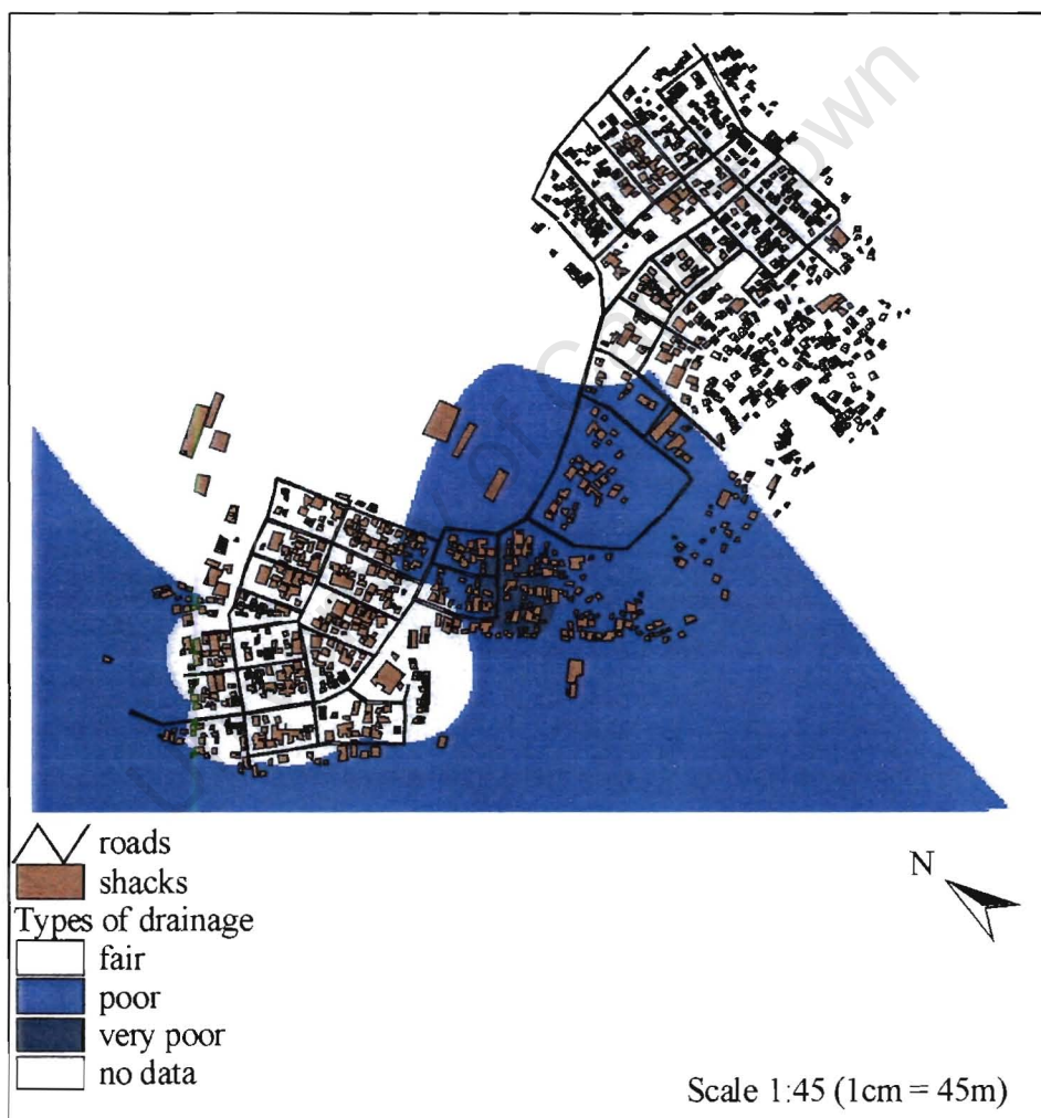
Figure 14. Drainage conditions in the settlement.
