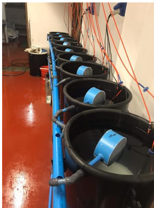
Figure 2: Nine black polyethylene cylindrical tanks were used to rear T. gratilla larvae, each fitted with a banjo sieve.
