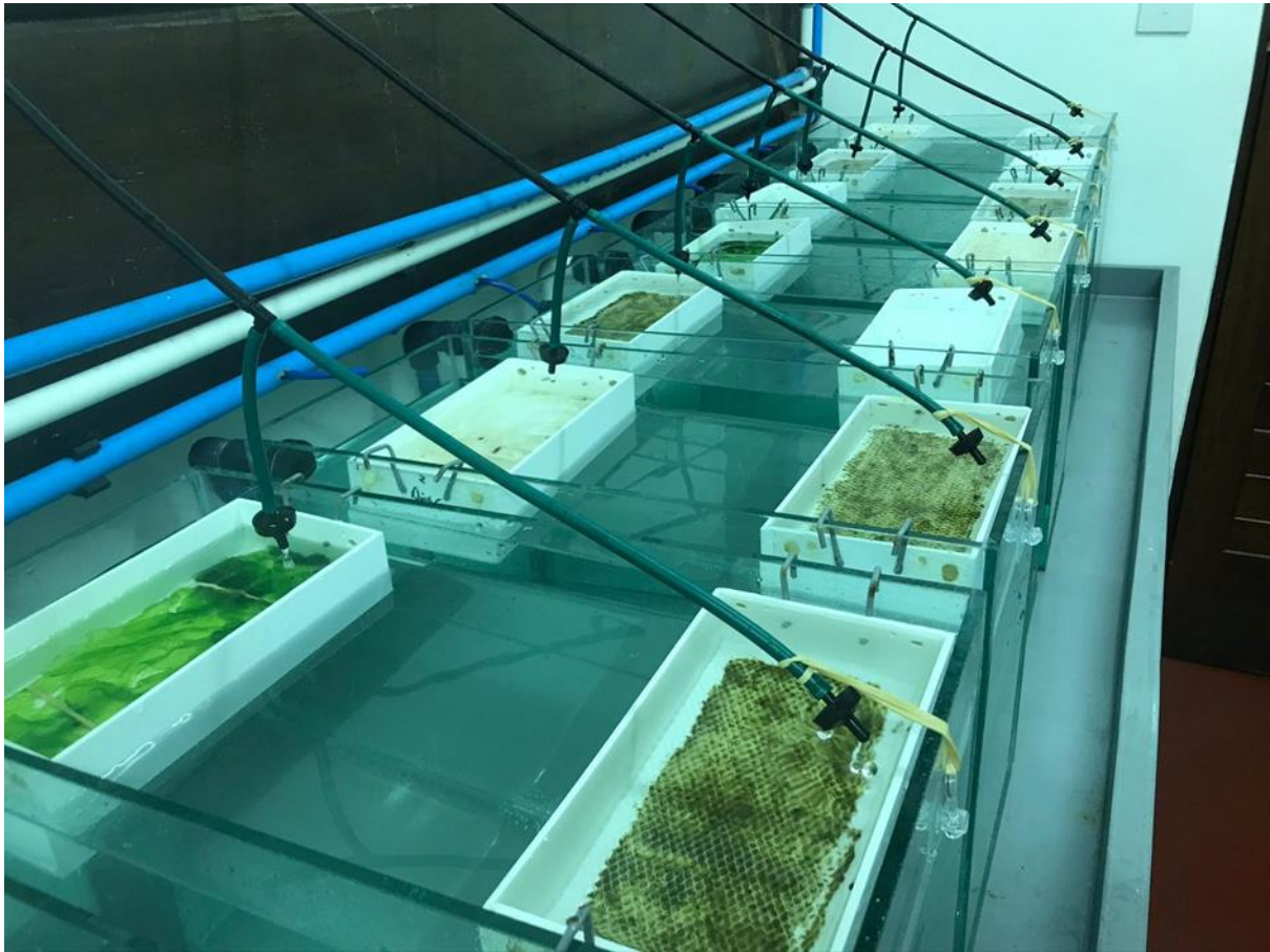
Figure 6: Each tank held two troughs suspended by PVC hooks in the water. Water drippers were held taut over each trough through with elastic bands.
