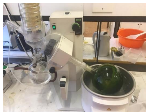
Figure 9: A Roto-Vap evaporator was used to evaporate off the solvents used during bulk extraction.
