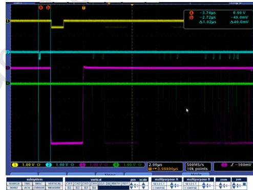
(b) analog Gate and delay generator delay measurement
