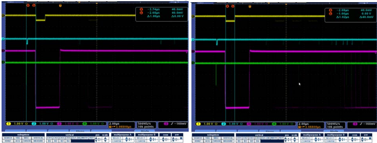
(c) Digital Gate and Delay generator delay measurement
