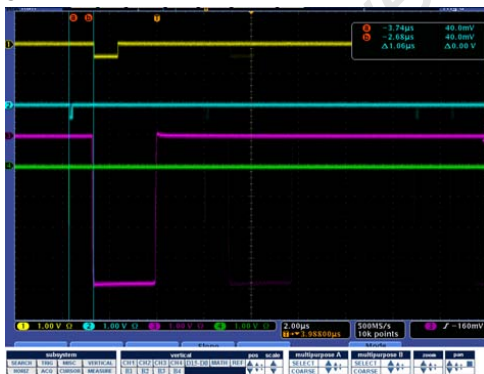
(c) digital Gate and delay generator delay measurement
