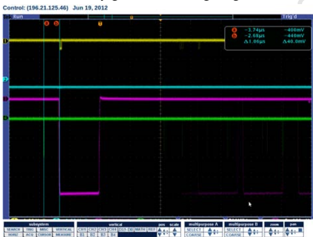
(c) Digital delay generator delay measurement
