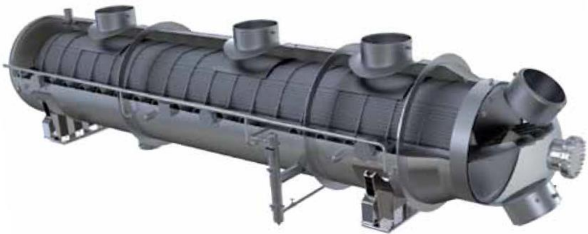
Figure 3-2. 3D image of a single zone horizontally mounted tube plate type FWH used on a nuclear power station [43]
