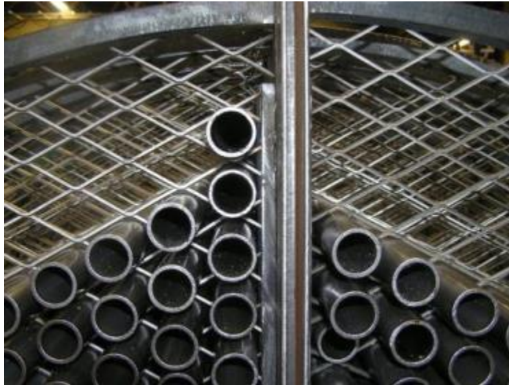
Figure 2-15. Tube arrangement in grid supports [20]
