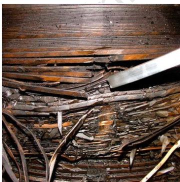
Figure 6-4: Inter turn Damage on HV Winding
