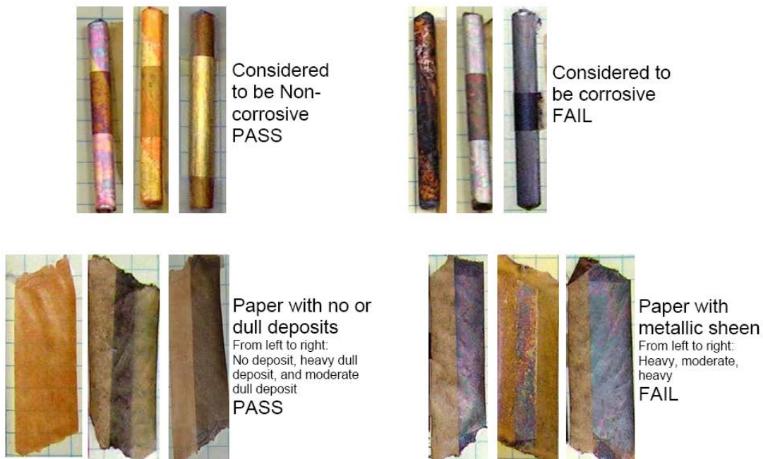
Figure 3-2: Copper Rods and Kraft paper insulation after testing [Lewand1]
