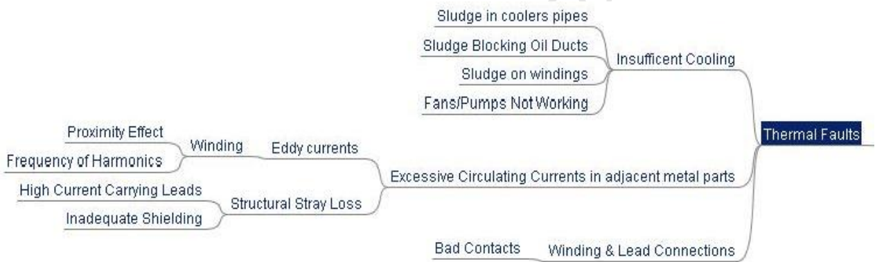
Figure 3-5: Origin of Thermal Faults in Power Transformers
