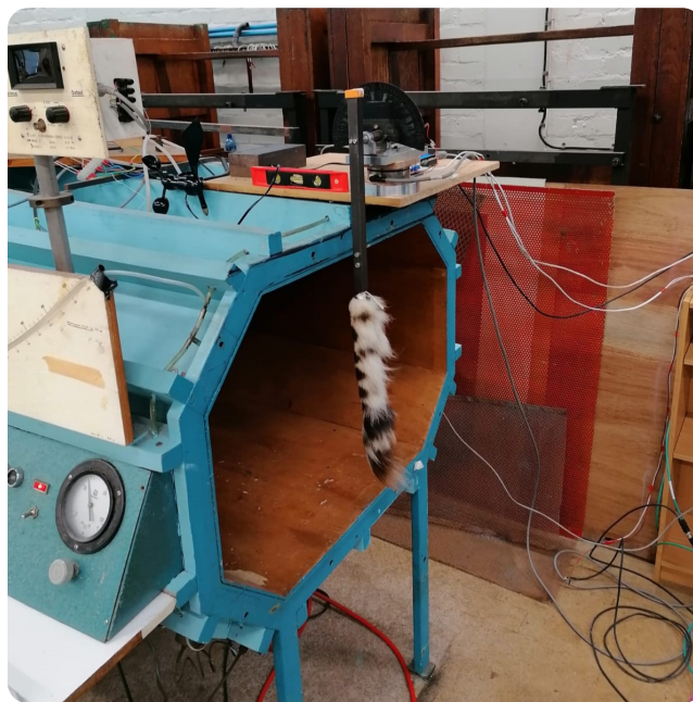
Figure 4.6: Wind tunnel test rig setup for the static procedures
