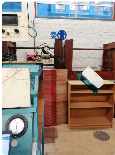
Figure 6.9: The wind tunnel rig with the tail attached. The tail is in a position such that sail end is in the wind.
