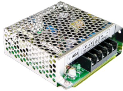
Figure 5.20: The SD-25B-12 DC-DC converter. Image taken from [54].
