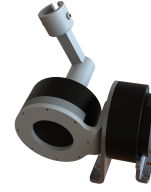
(d) Fourth concept design using two AK70-10 T-Motors with no external gearing.
