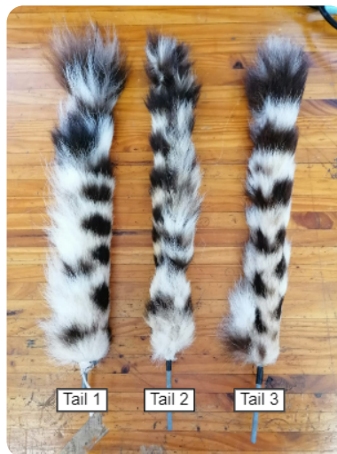
Figure 4.2: The three tails used in the wind tunnel experiment to determine the aerodynamic characteristics of the cheetah's tail. The tails from left to right are tails 1, 2, and 3, respectively.
