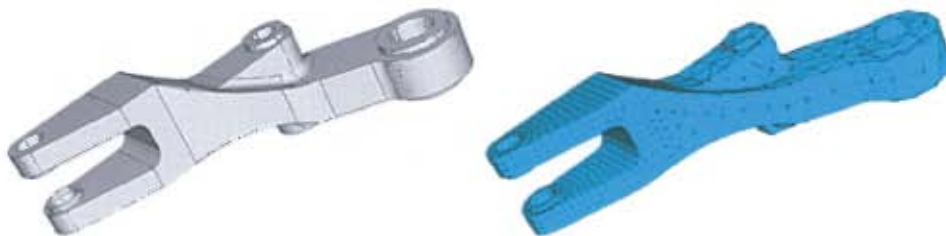
Figure 5.1: Discretisation of a solid into elements and nodes
