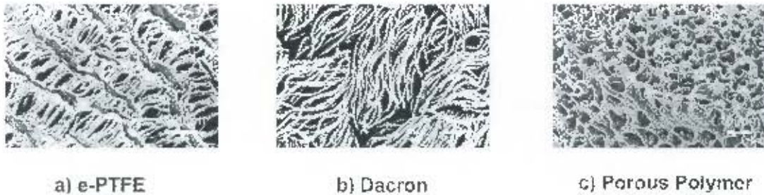
Figure 2.12: Various synthetic graft micro-structures
