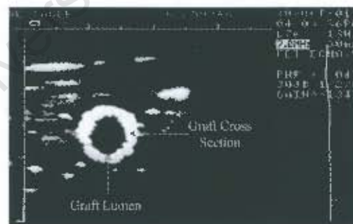
Figure 7.12: Ultra-sound image of porous graft cross-section showing distorted image due to trapped air in micro-porous structure
