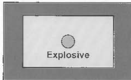
Figure 2.16: Illustration of fully confined blast loading
