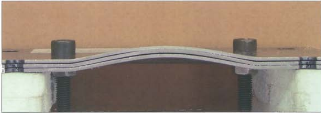
Figure 4.10: Photograph of plate profile for test plate subjected to same charge mass (5g) but different load conditions (LC-1, LC-2 and LC-3) Test plate Numbers, NJ210405a, NJ210405b, NJ210405c
