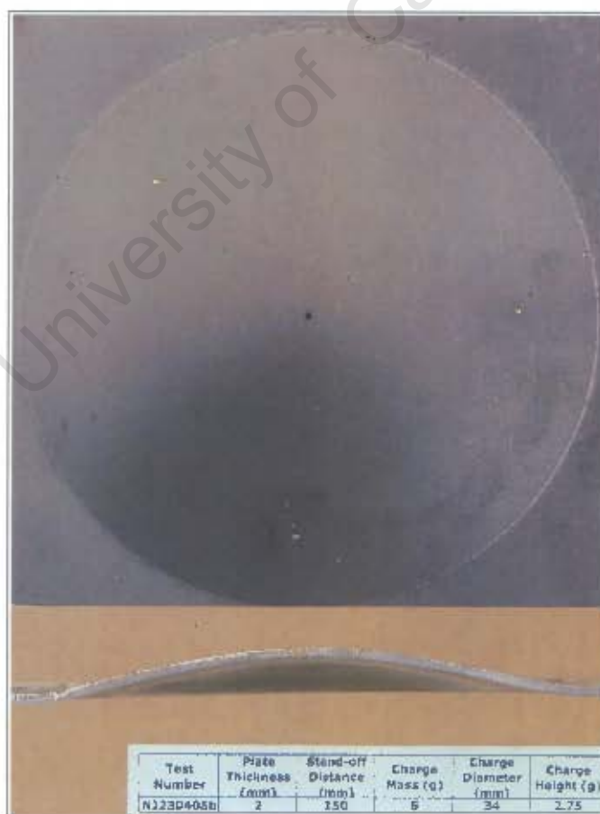
Figure 4.1: Photograph of plate profile showing large global dome. Plate number NJ230405b, I = 12.03Ns , S = 150mm
