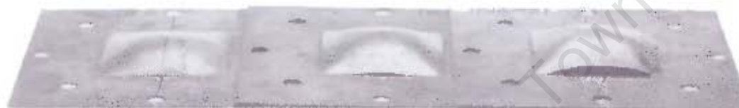
Figure 2.36: Increasing mid-point deflection for increasing impulse with partial tearing along plate boundary [4]
