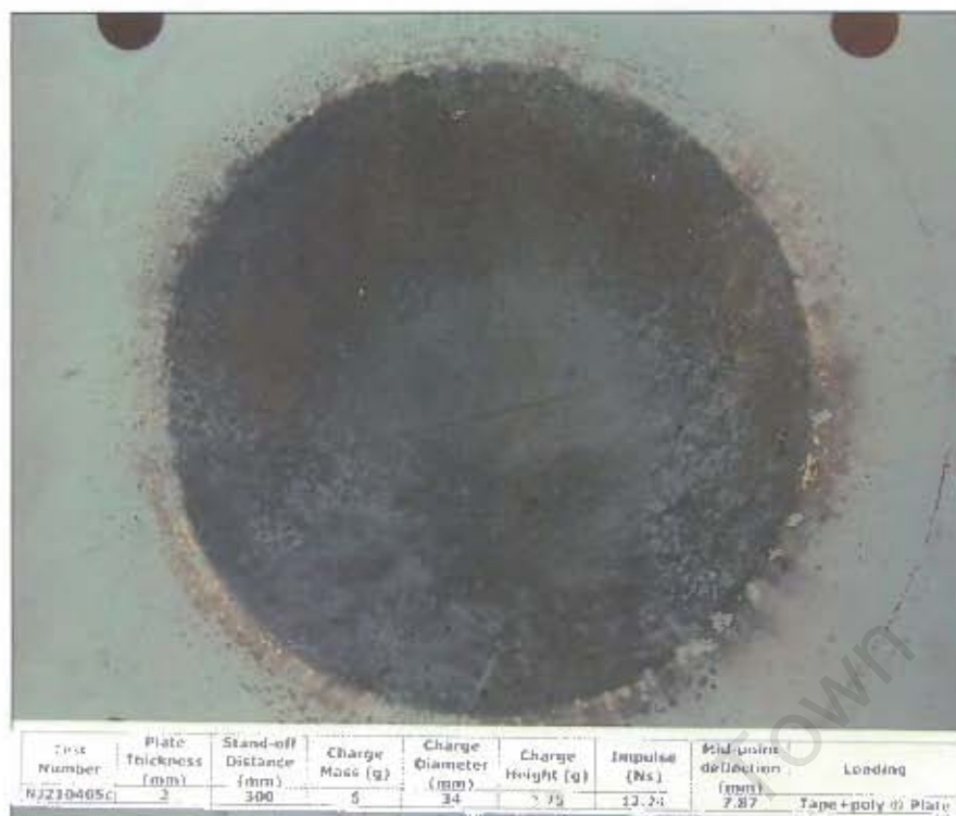
Figure 4.8: Photograph of polystyrene residue visible for test plate subjected to load condition LC-3
