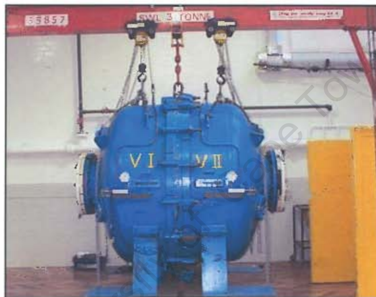
Figure 2.33: Photograph of pressure pulse loading rig [24]
