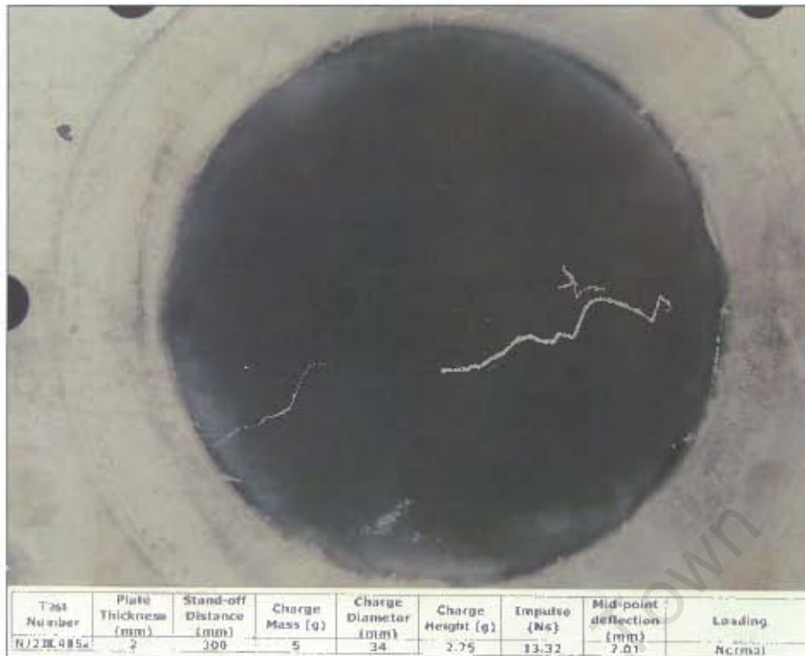
Figure 4.6: Photograph of black soot observed for test plate subjected to load condition LC-1 Test plate Number NJ210405a, S = 300\text{mm} , I = 13.32\text{Ns} and Mid-point deflection = 7.01\text{mm}
