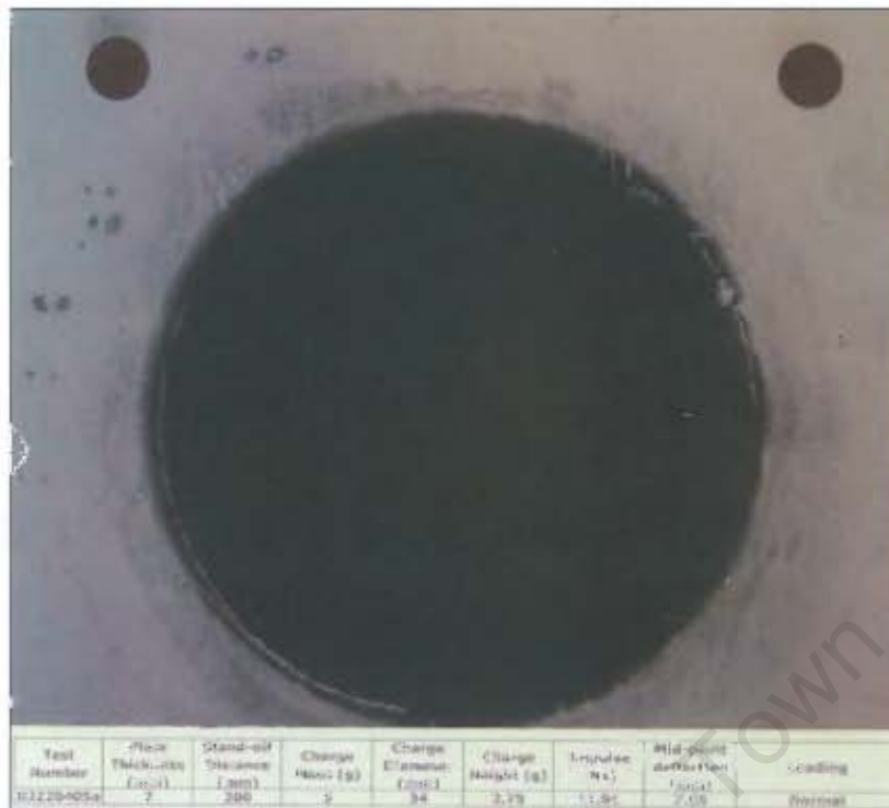
Figure 4.13: Photograph of uniform coat of soot, no visible indication of burn diameter for test specimen NJ220405a, S = 200\text{mm} , charge mass 5\text{g} , I = 11.91\text{Ns} , Load condition LC-1
