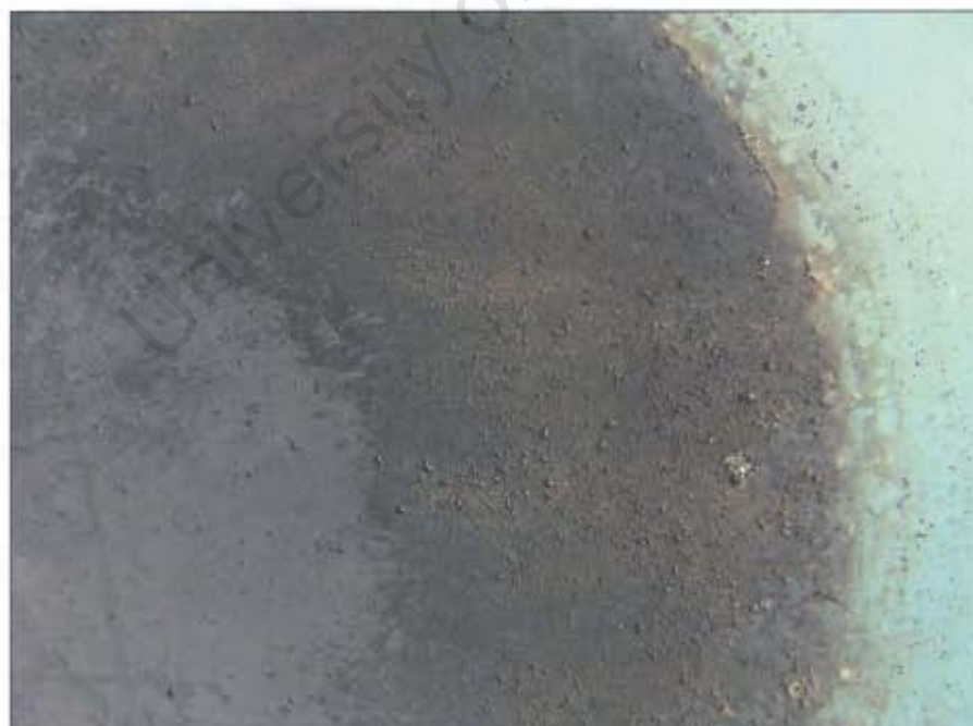
Figure 4.9: Photograph showing a close up view of the polystyrene residue visible for test plate (NJ210405c) subjected to load condition LC-3
