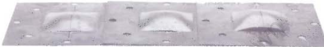
Figure 2.45: Increasing mid-point deflection for increasing impulse with partial tearing along plate boundary [4] (repeated figure)
