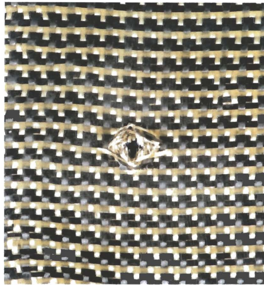
Figure 4.56 Mixed ductile /brittle surface damage on the bottom surface of the carbon / Kevlar ® hybrid impacted specimen at approximately 6 J.
