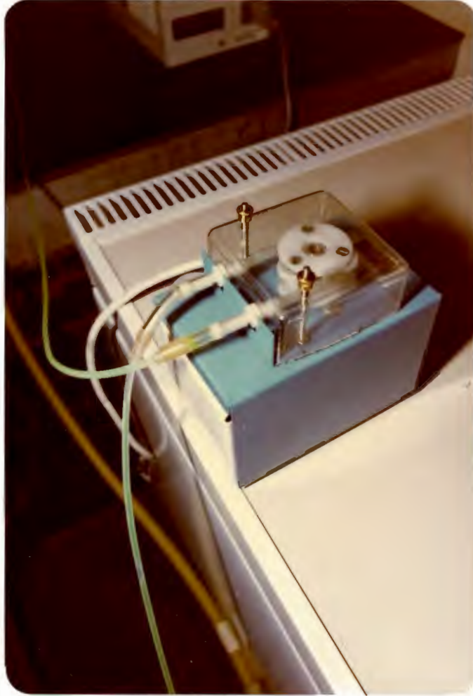
Fig. 12 Peristaltic pump for pumping antifreeze through the cooling system. The flow rate was controlled by means of a clamp.
