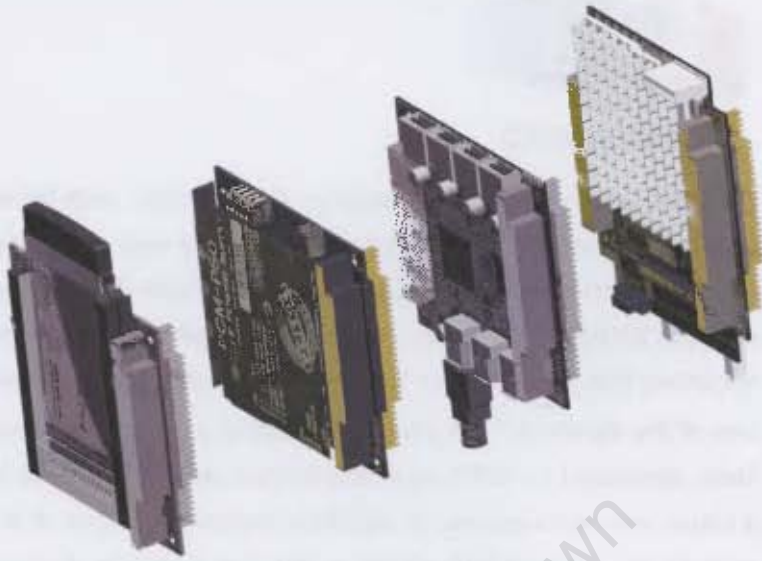
FIGURE 2-11: DGPS: POWER SUPPLY AND SBC
