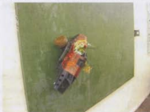
FIGURE 5-1: TESTING OF VEHICLE ON A VERTICAL FERRO-MAGNETIC BOARD
