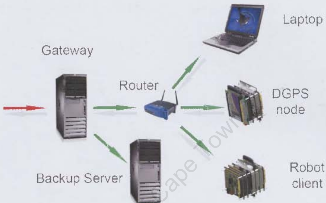
FIGURE 4-11: FULL LAN ARCHITECTURE
