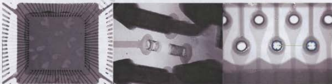
FIGURE 1-1: X-RAY INSPECTION OF ELECTRONIC COMPONENTS AND PCB 'S
