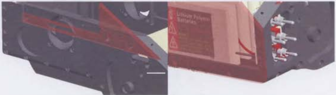
FIGURE 3-19: FRAME WEIGHT REDUCTION (LEFT) AND BATTERY INSERTS (RIGHT)
