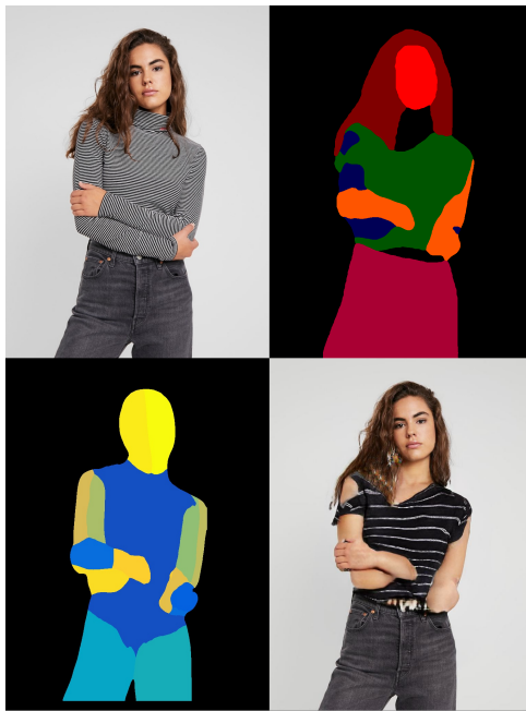
Figure 5.7: An example highlighting the limitations experienced by the off-the-shelf models when dealing with complicated poses. Shown at the top left is the target person image, with the resulting segmentation map found by PGN shown at the top right. The dense correspondence, found with Densepose, can be seen at the bottom left, while the resulting virtual try-on can be seen at the bottom right.
