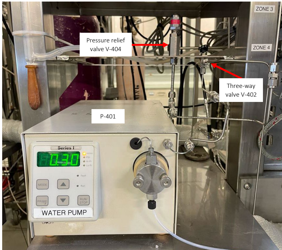
Figure A-10: Lab Alliance Series I HPLC pump P-401 to control the liquid water flowrate
