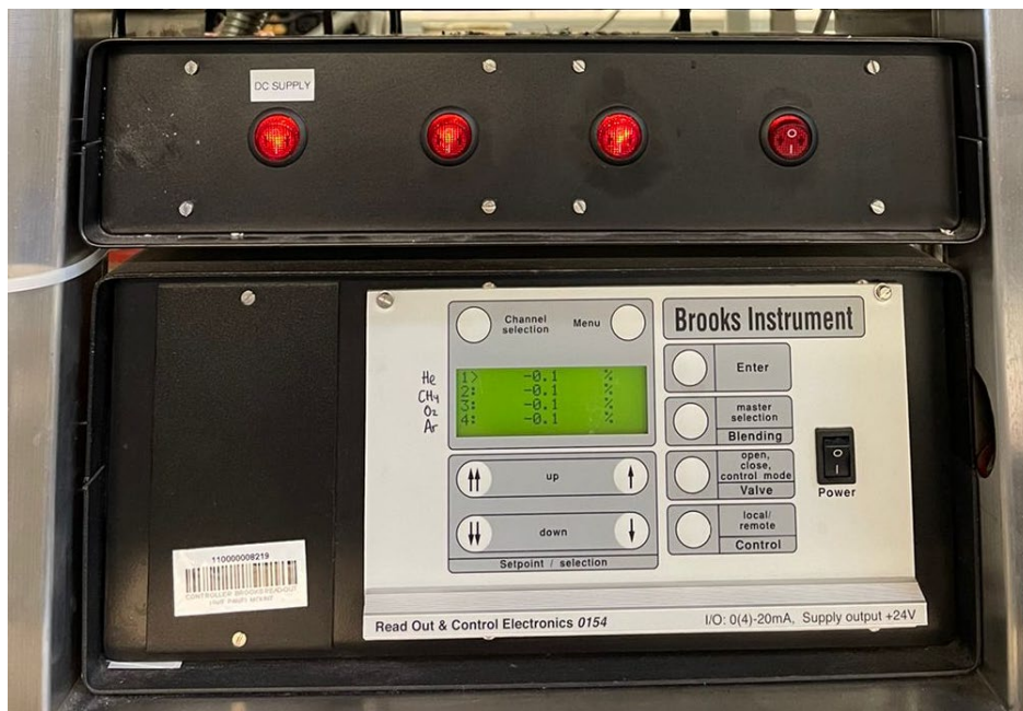
Figure A-4: Four-channel Brooks flow control module for methane, oxygen, helium and argon
