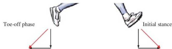
Figure 2.30.: Interaction forces between a runner and a footbridge. (Occhiuzzi et al. , 2008)
