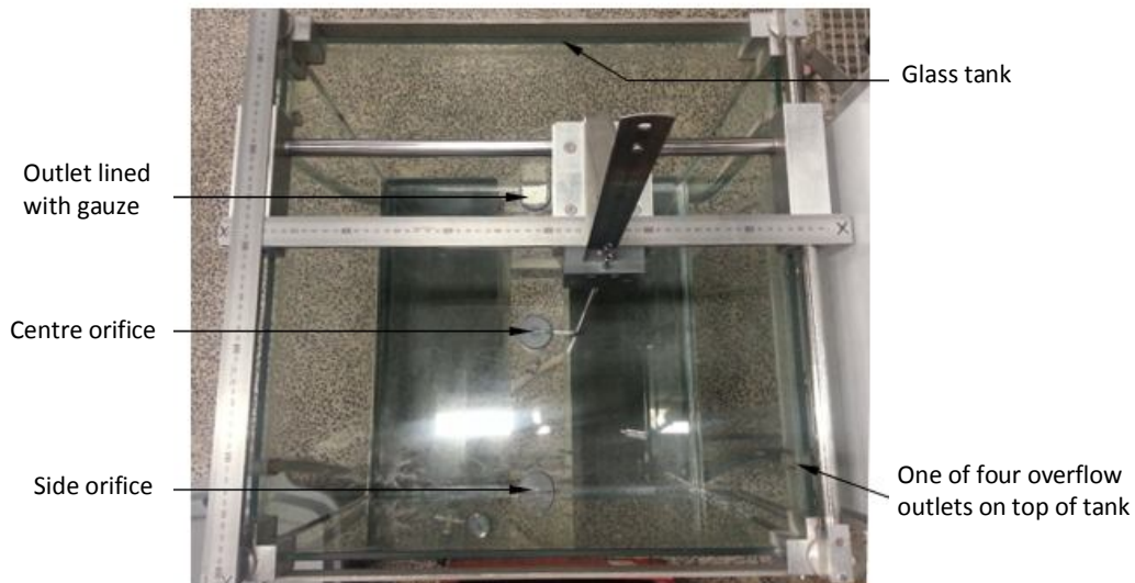
Figure 3.1: Plan view of the experimental setup showing components of the tank
