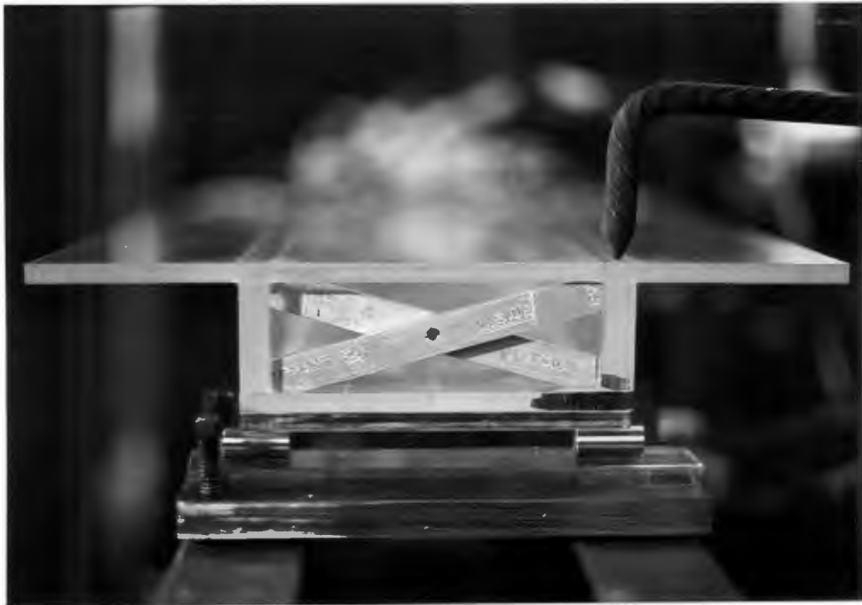
Plate 2 Roller support details.
