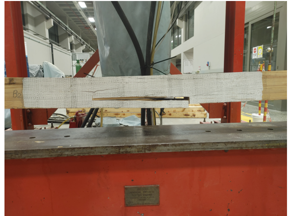
Figure 10.29: Beam B2 global strain vs failure point, 0.5s before failure
