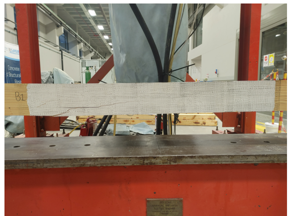
Figure 10.28: Beam B1 global strain vs failure point, 0.5s before failure
