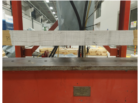
Figure 10.32: Beam B5 global strain vs failure point, 0.5s before failure
