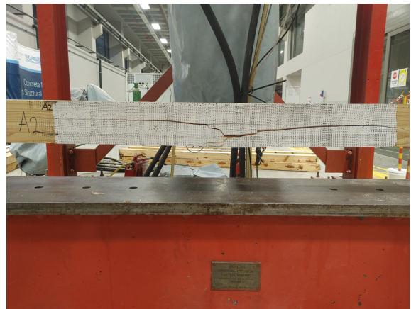
Figure 10.24: Beam A2 global strain vs failure point, 0.5s before failure
