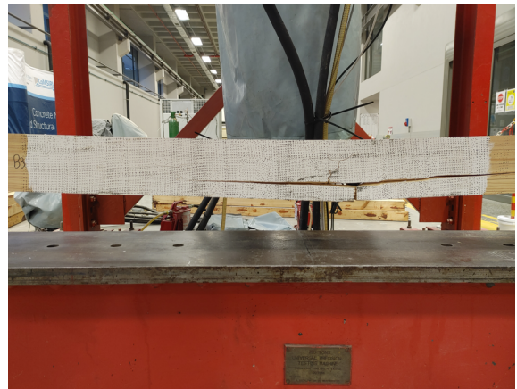
Figure 10.30: Beam B3 global strain vs failure point, 0.5s before failure
