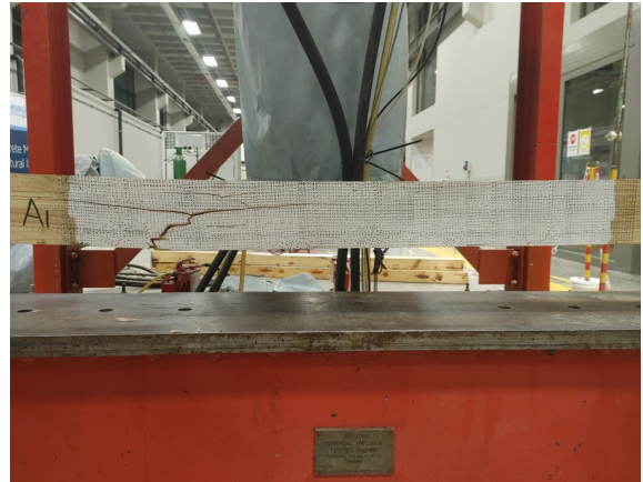
Figure 10.23: Beam A1 global strain vs failure point, 0.5s before failure
