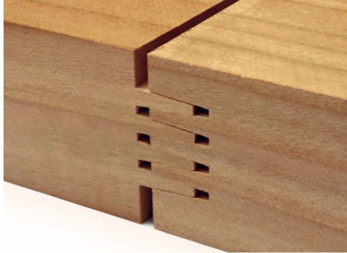
Figure 2.15: Typical finger joint used in glulam production, before adhesive application
