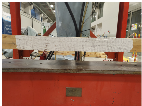
Figure 10.31: Beam B4 global strain vs failure point, 0.5s before failure
