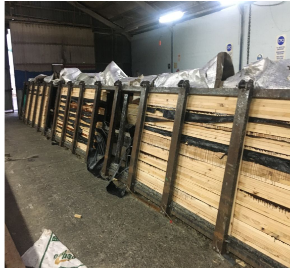
(b) Beams in the 50T press while curing
