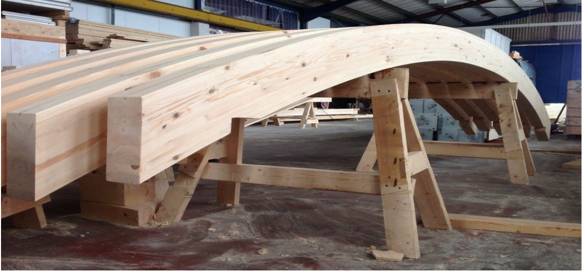
Figure 3.3: cambered glulam beam in the factory
