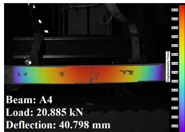
Figure 10.5: Beam A4 at 10 kN and 0.5s before failure
