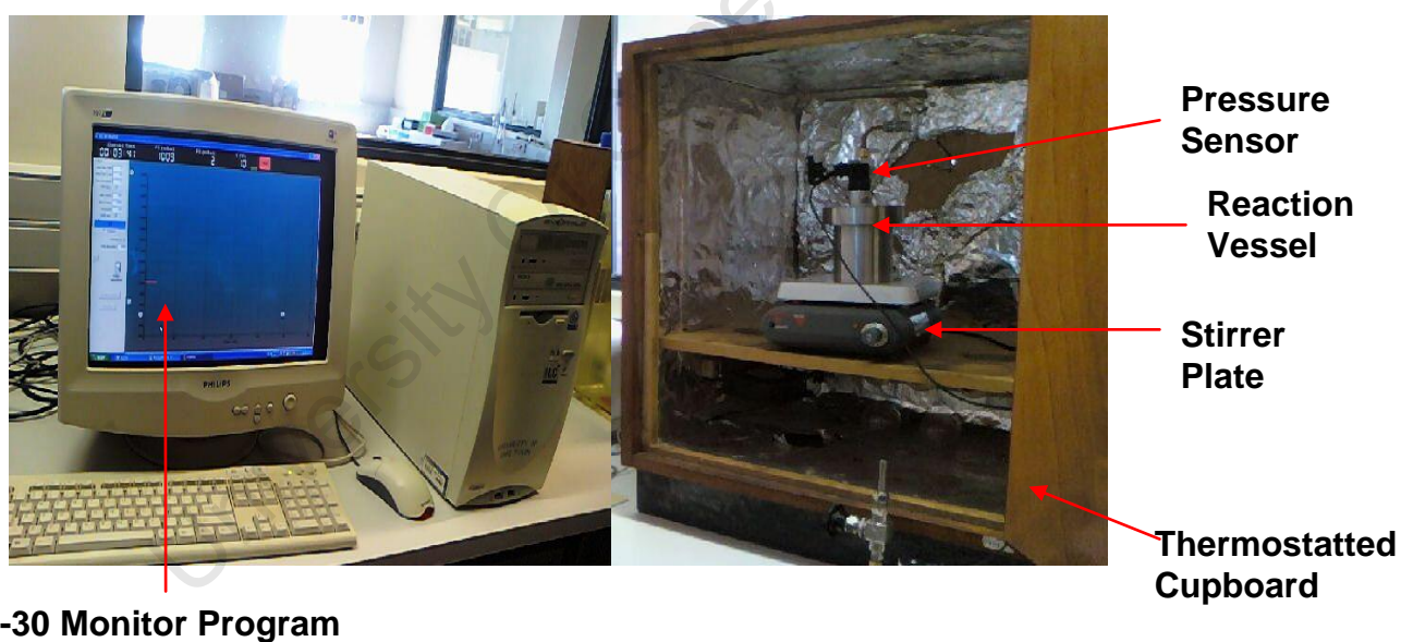
Figure 2.1: Illustration of the apparatus/experimental set up for the ammonium nitrate-sodium nitrite reaction
