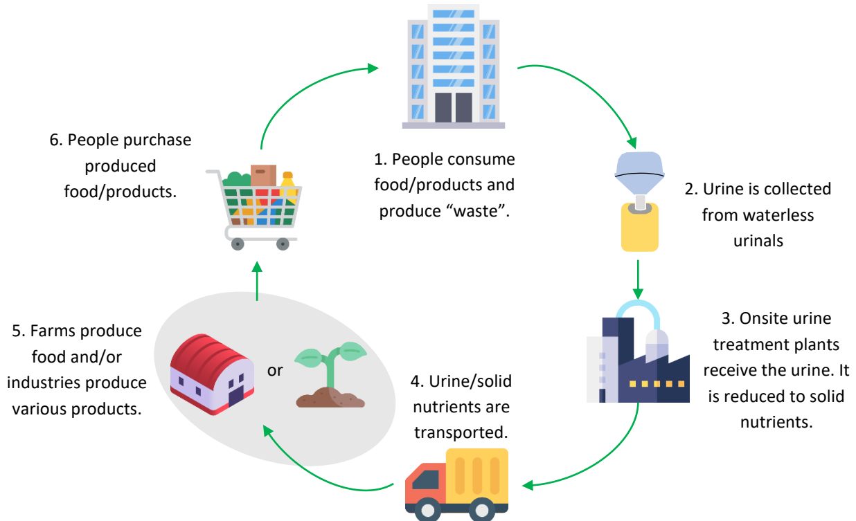
Figure 1-1: A conceptual visualization of a closed loop cycle where "wastes" are reimaged as valuable nutrients for ensuring food security and producing value-added products.
