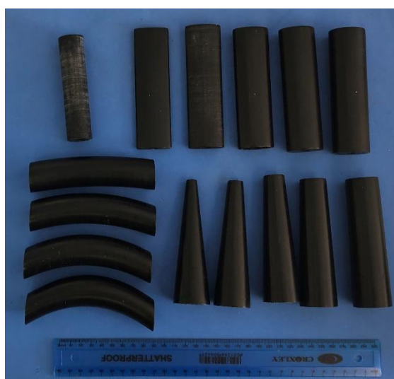
Figure 2-12 3D printed conductive PLA idealised geometry mandrels to model geometric features of patient-specific graft geometry
