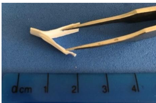
Figure 2-25 A force-delaminated electrospun graft scaffold sample
