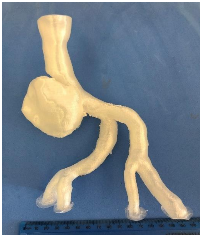
Figure 2-27 3D printed P16 transparent PLA aortic model
