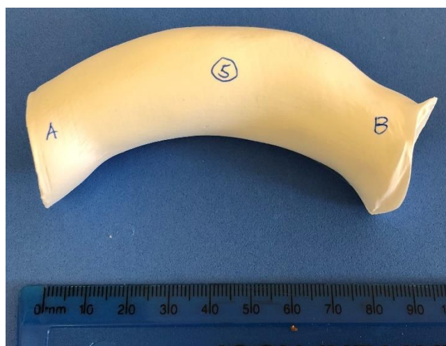
Figure 3-16 Electrospun Pellethane graft scaffold, on patient-specific P16 graft geometry
