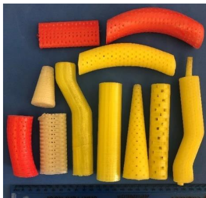
Figure 2-6 3D printed non-conductive PLA mandrels
