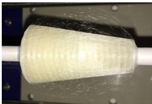
Figure 3-6 Minimal electrospun fibres around non-conductive PLA mandrel (1 mm perimeter holes)
