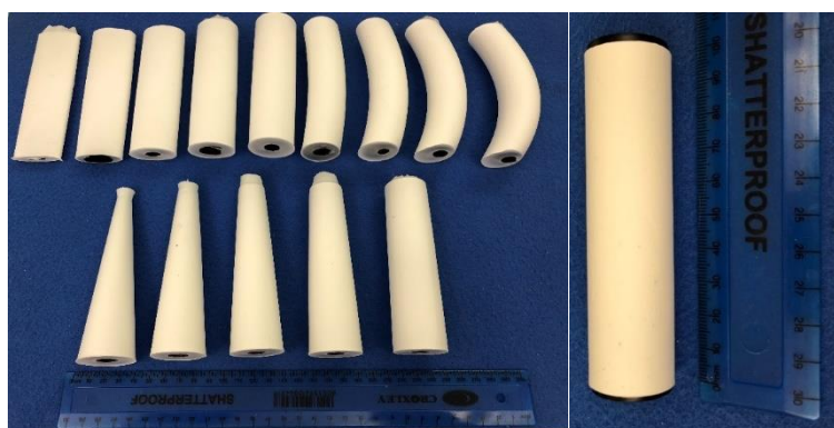
Figure 3-12 Electrospun graft scaffolds on 15 idealised geometry 3D printed conductive PLA mandrels
