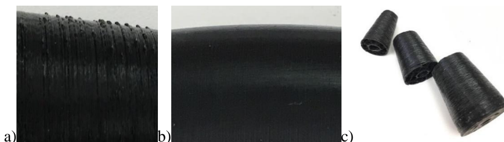
Figure 3-7 a) untreated surface of 3D print (0.1 mm layer height), b) treated surface of 3D print (sanded & vapour smoothed), c) broken mandrel due to excessive vapour smoothing
