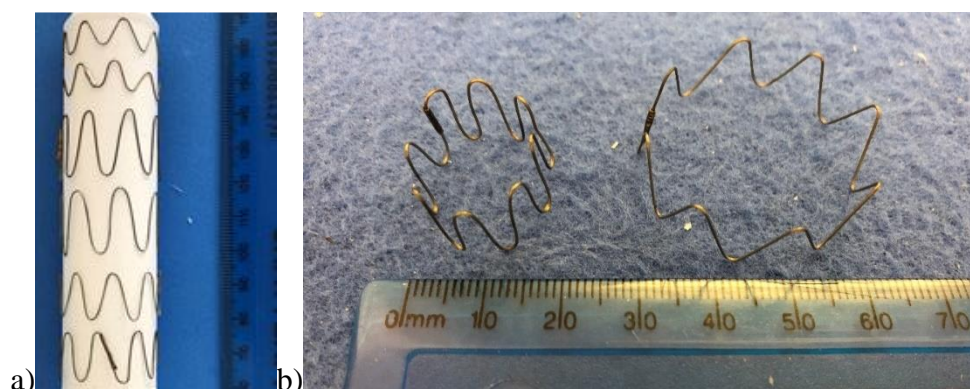
Figure 3-33 a) various Nitinol stent patterns after heat-set, b) crimped and expanded body temperature Nitinol stent ring at room temperature
