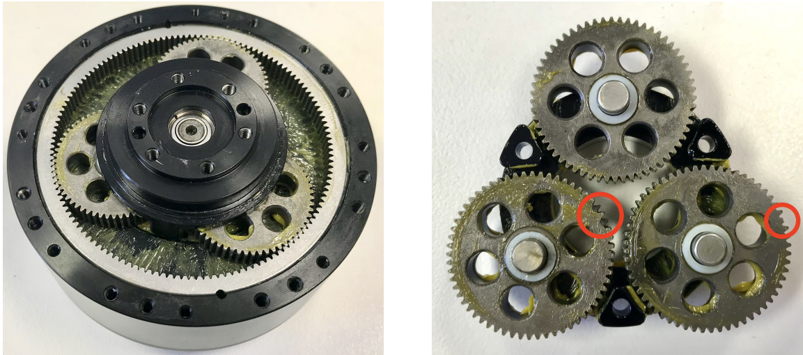
Figure 2-10: AK70-10 planetary gearbox with front cover removed (Left), and exposed planet gears on carrier with their steel dowel pins, nylon spacers, and broken gear teeth circled in red (Right).
