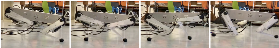
Figure 4-6: Several frames of Kemba bounding to the right at 1.5 m/s. Frames show a full gait cycle. From left to right; front foot touchdown and stance phase, rear foot touchdown, front foot lift-off and rear foot stance phase, rear foot lift-off and extended flight phase.
