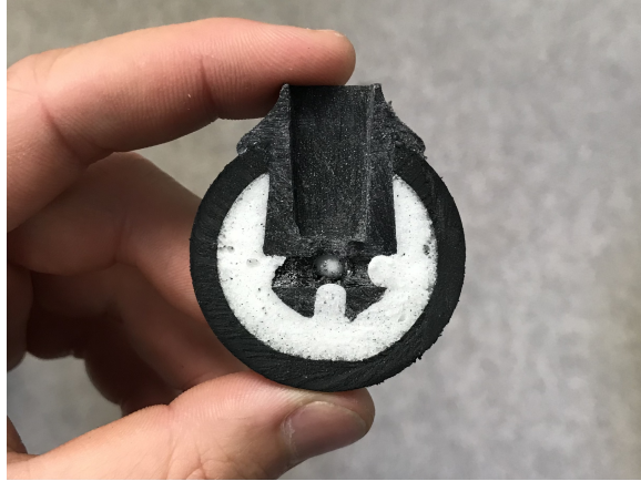
Figure 2-12: Squash ball foot cut in half exposing functional layers and 3D printed insert. Holes in the insert provide a place for excess foam to expand.
