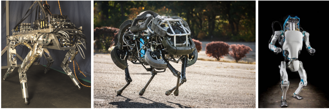
Figure 1-2: Hydraulically actuated robots HyQ [4] (Left), WildCat (Middle), and Atlas (Right) [3].
