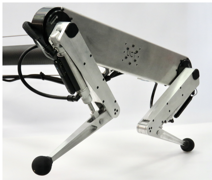
Figure 2-1: Kemba, a hybrid pneumatic and electric actuated legged robot.
