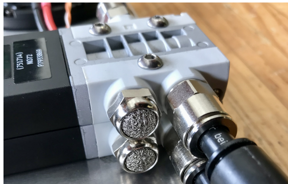
Figure 2-8: Stacked solenoid valves with vent port mufflers.
