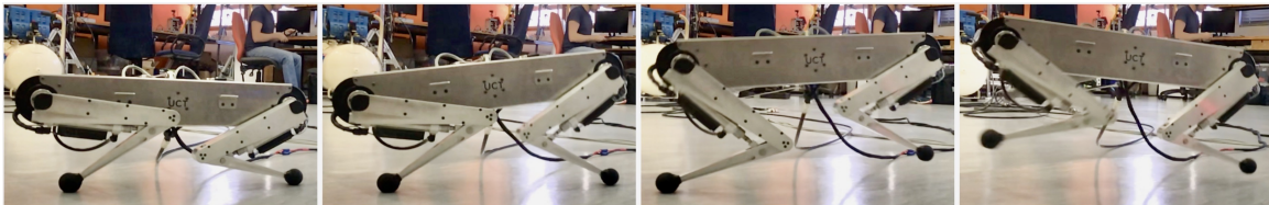
Figure 4-12: Several frames of Kemba accelerating from rest into a 1.5 m/s bound. Frames show the full 0.5 s acceleration motion. From left to right; set pose, front foot popup, rear foot push-off, extended flight phase.
