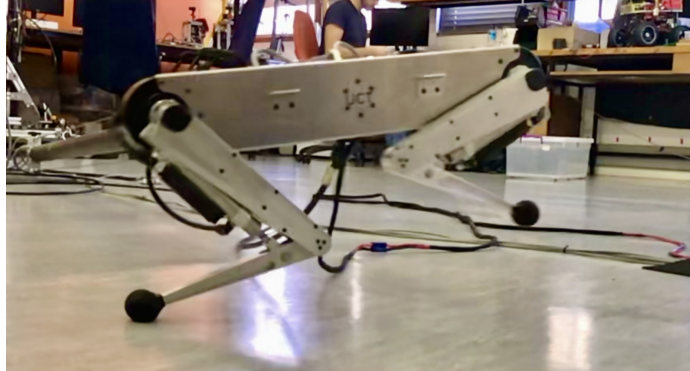
Figure 1-1: A photo of Kemba pushing off of with its hind leg and accelerating into a 1.5 m/s bounding gait.
