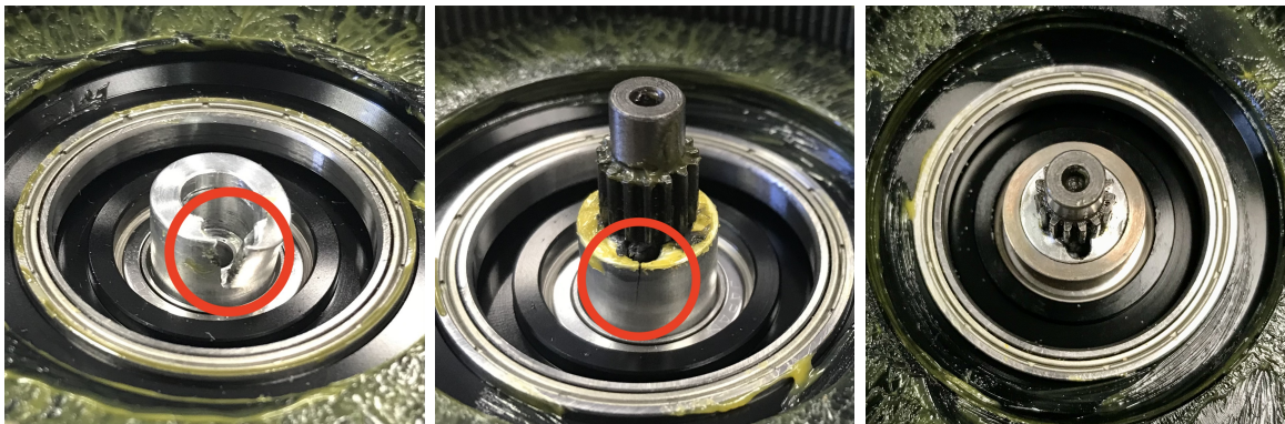
Figure 2-9: AK70-10 sun gear failure showing torn open pin slot (Left) and hairline crack developing in the same position on the second motor (Middle). Press fit steel collar to reinforce pin slot (Right).
