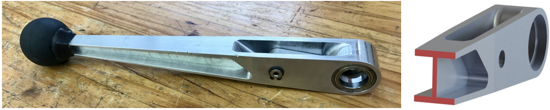
Figure 2-4: Tibia with press fit bearings and foot (Left) and section view showing I-beam cross section (Right).
