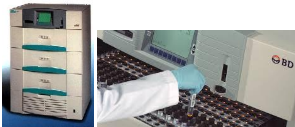
Figure 11. Mycobacterial Growth Indicator Tube (MGIT) machine and technologist loading machine with MGIT tube. (209)
