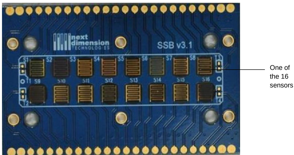
Figure 6. Image of the sixteen sensors of the test device. (Image courtesy of Dr Will Royea, NextDimension Technology)
