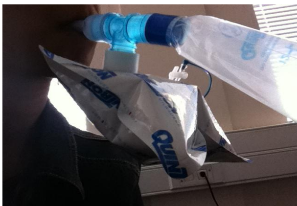
Figure 9. Researcher exhaling into bag showing the full reservoir bag and breath collection bag slowly inflating.
