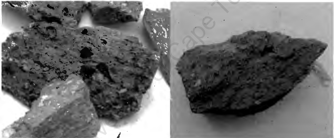
Figure 7.12: Flakey, honeycombed and porous surface of the NFX RA compared to FBE45 RA
