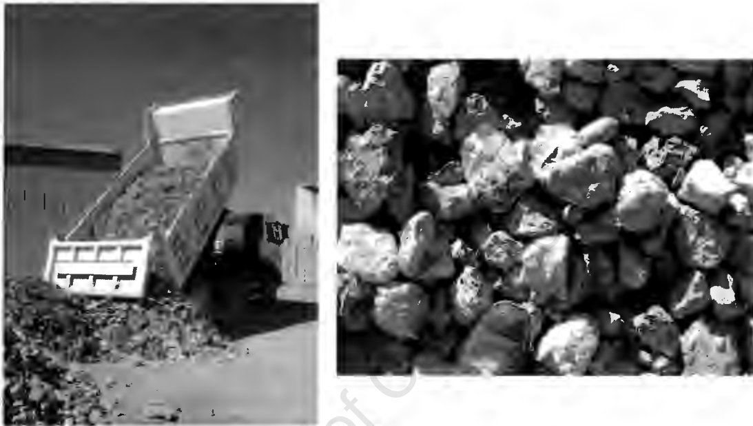
Figure 6.7: (Left) RCA materials being delivered to CapeBrick for storage and use in the manufacture of concrete masonry elements. (Right) Pre-crushed RCA used in this study
