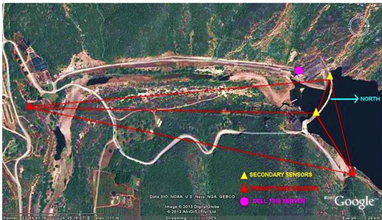
Figure 7.9: Kouga Dam GNSS/GPS Network (adopted from Pretorius & du Toit, 2014)
