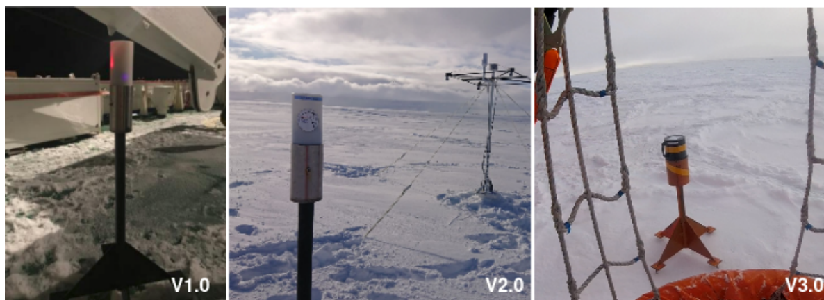
Figure 1.4: SHARC Buoy Versions shown during the various deployments. From left to right, SHARC Buoy V1.0 deployed on deck before final deployment during the SCALE winter cruise 2019, V2.0 deployed during the summer 2020-2021 Polarstern expedition in the Weddell Sea and V3.0 immediately after a basket deployment during the SCALE winter cruise 2022.
