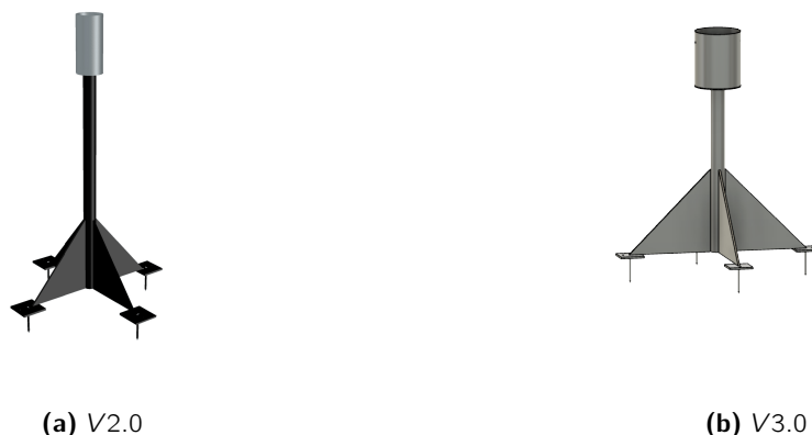
Figure 5.1: Changes in stand design between SHARC Buoy V1.0 and V3.0 Design credit: V2.0 Keith MacHutchon, Robyn Verrinder, V3.0 James Hepworth
