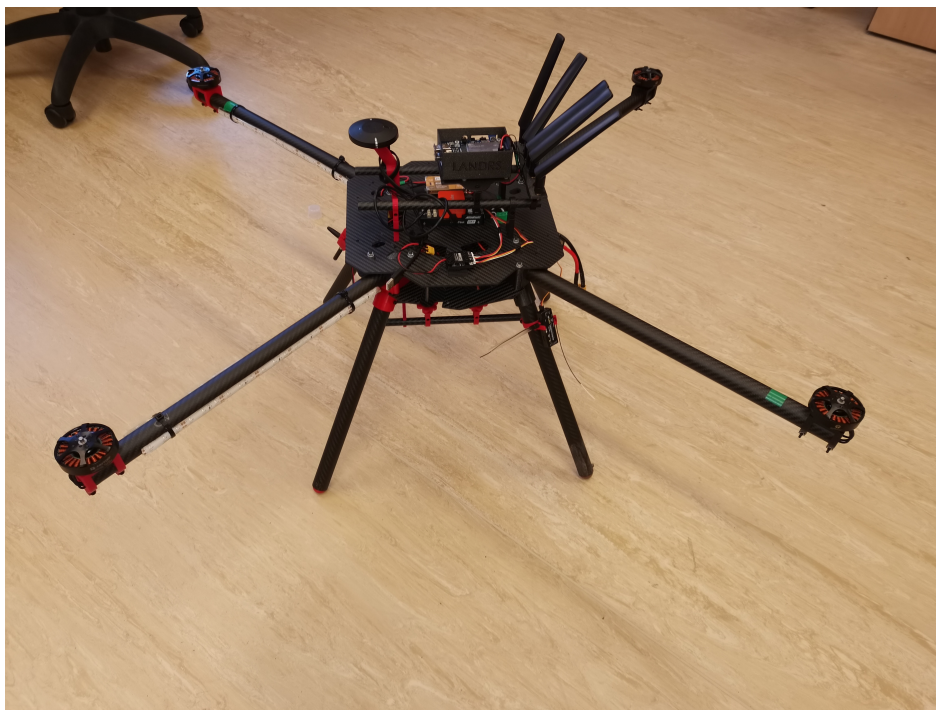
Figure 3.11: Landrs Nyala Hexaquad drone used for experiments (In quad-rotor configuration)
