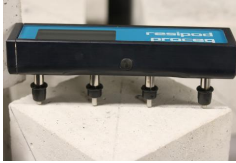
Figure 3.8: Surface resistivity test with a 4-point probe on a 150-mm cube
