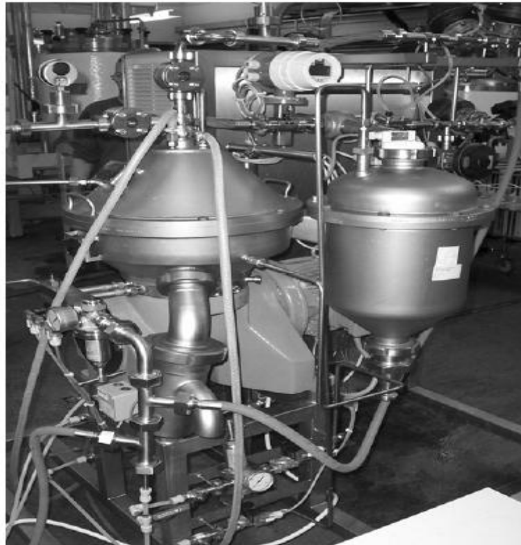
Figure 2-3: The pilot brewery 5 hl.l -1 disk stack centrifuge (Stewart et al. 2006).
