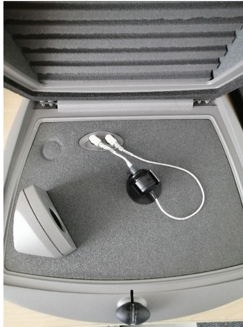
FIGURE 8. COUPLER MICROPHONE CALIBRATION SET UP
