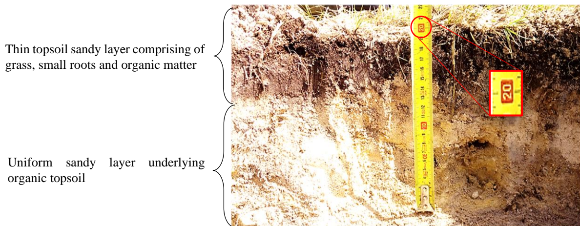
Figure 4-3: Surface strata observation pit in a pond from surface to 20cm depth
