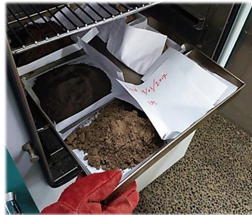
Samples removed after 24 hrs to be used for sieve analysis and specific gravity test
