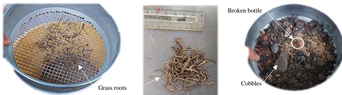
Figure 5-5: Organics, impurities, and cobbles removed from samples before sieve analysis
