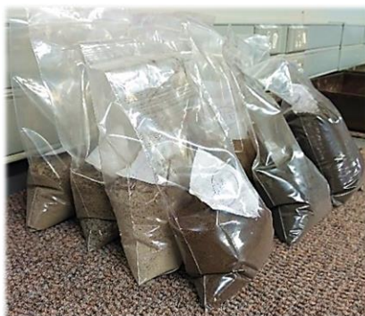
Dry soil samples in sealed plastic bags to mitigate change in moisture content
