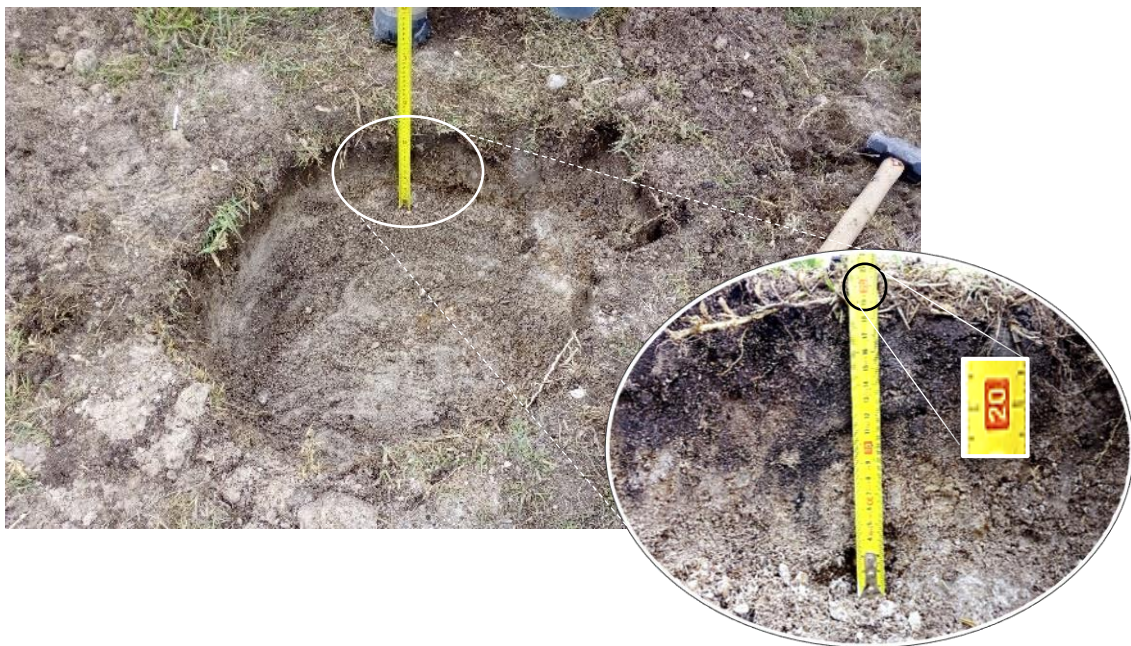
Figure 4-13: Preparation of sub-surface DRI test
