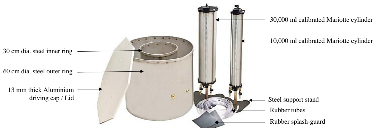
Figure 4-8: Double-Ring Infiltrometer Apparatus
