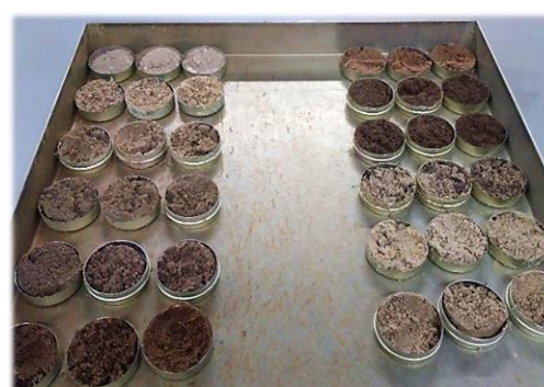
Oven-dried samples in small tins for determination natural moisture content
