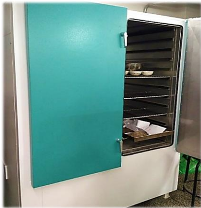
Laboratory oven used to dry soil samples at 105°C
