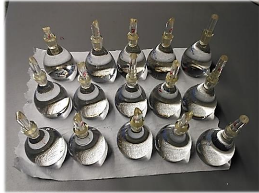
Small pycnometer bottles with distilled water only.
